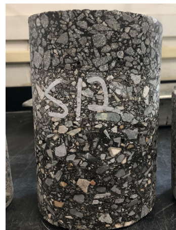
Figure 12. Core from Section S12 with HMA over CCPR base.
