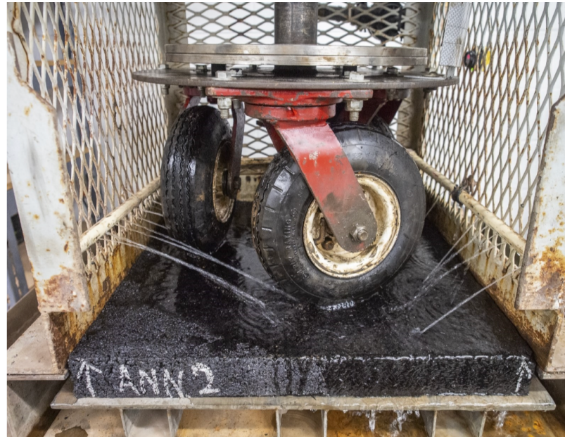
Figure 11. NCAT Three Wheel Polishing Device.
