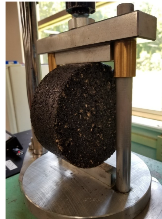
Figure 2a. High-Temperature IDT (HT-IDT) Test
