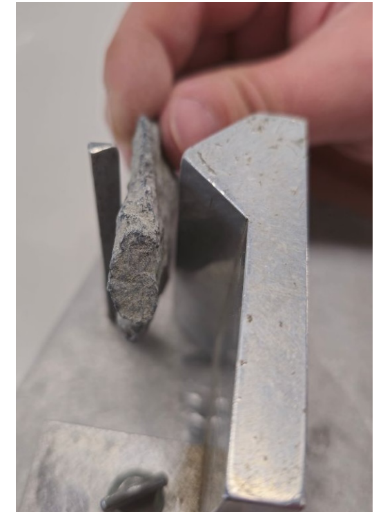
Figure 7. Flat and Elongated test and apparatus.
