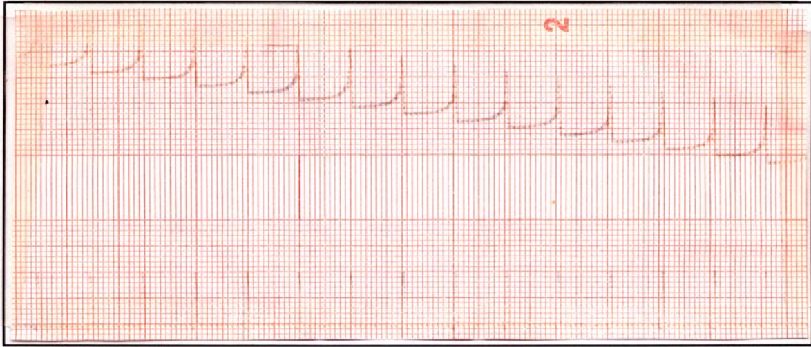
Figure 3. Typical Recorder Output of a Resilient Modulus Test
