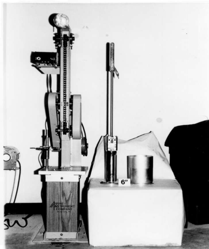
Figure 2. Compaction Equipment for 4" and 6"- Diameter Specimens
