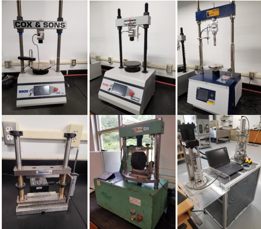
Figure 2: Devices used in study (from left to right): Top row: Cox & Sons 9500, Humboldt 5125, InstronTek Auto-SCB. Bottom Row: InstronTek Smart-Jig, Pine 850T (with InstronTek Smart-Jig), and Troxler IDEAL Plus
