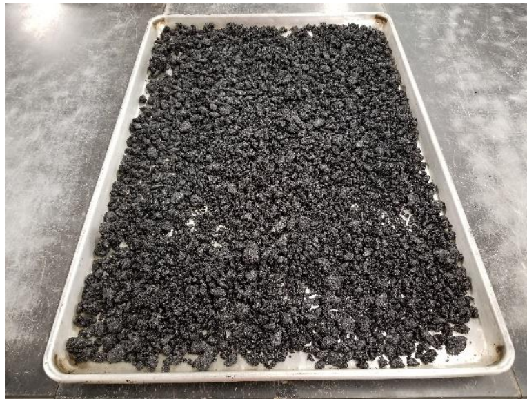
Figure 1. Mix in a Thin Layer for Critical Oven Aging
