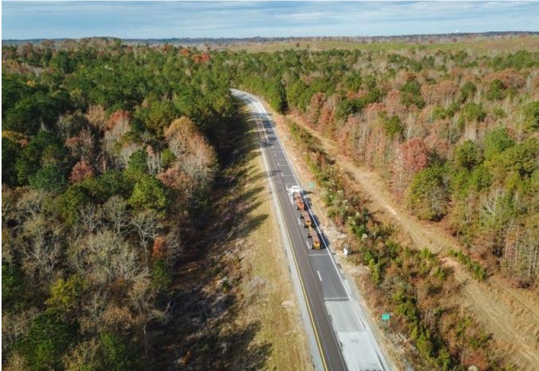
Figure 3. Heavily Loaded Triple-Trailer used for Accelerated Loading on the Test Track
