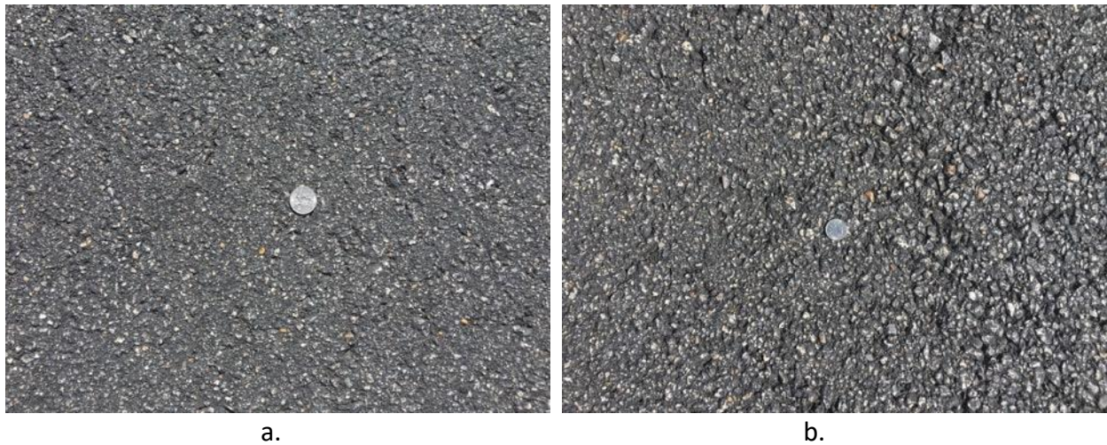
Figure 18. Difference in Surface Texture of (a) Section E5A (93.6%) and (b) Section E6A (87.9%)
