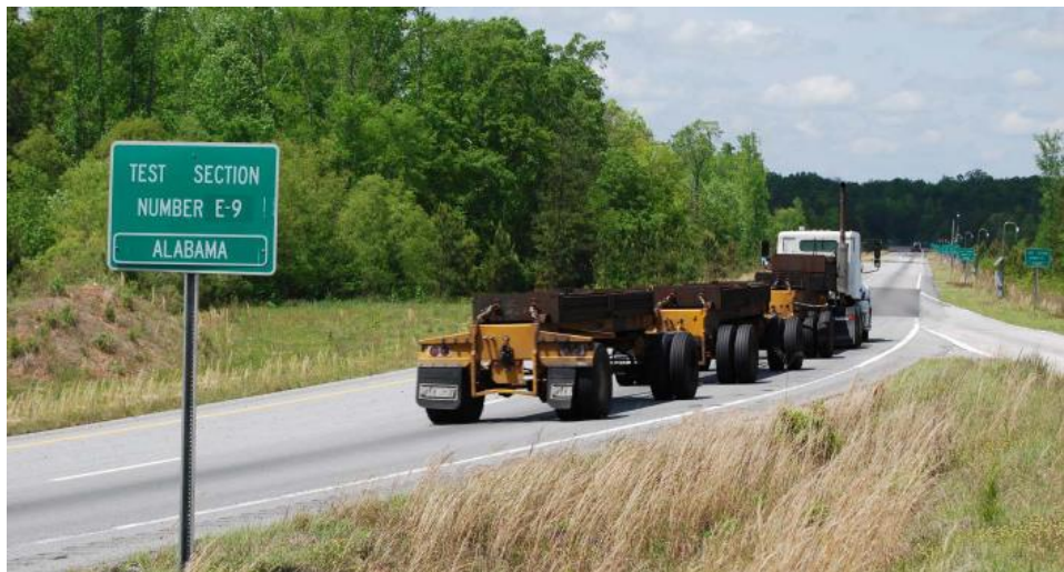
Figure 32. Heavily Loaded Triple-Trailer on the NCAT Test Track
