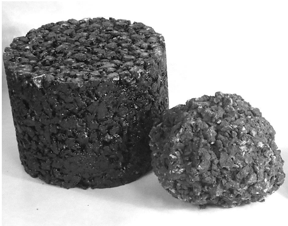
Figure 10. Before and After Cantabro Test Results
