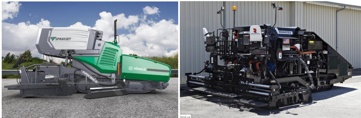
(a) (b) Figure 17. (a) Vögele SprayJet Paver and (b) Roadtec SP-200 Spray Paver
