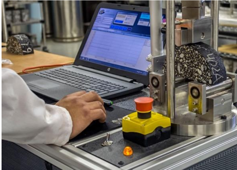
Figure 10 Test Quip® I-FIT Device
