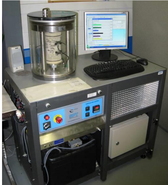
Figure 1 IPC Global Asphalt Mixture Performance Tester
