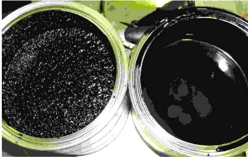
Figure 13 Asphalt Rubber Binder (left) and Terminal Blend Binder (right) (70)
