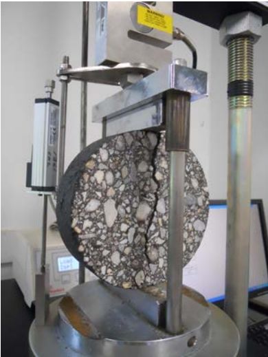
Figure 5. IDT Test Setup and Specimen Configuration
