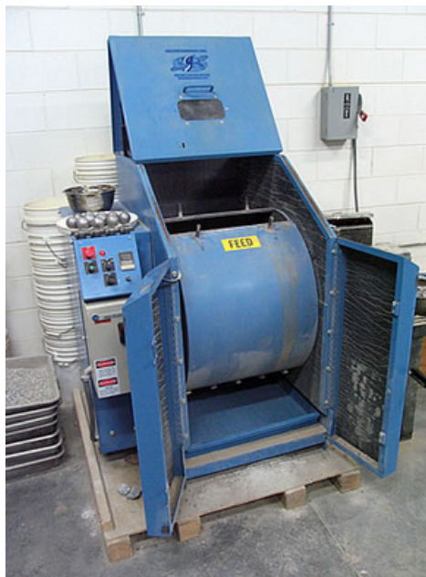
Figure 6 L.A. Abrasion Testing Equipment (7)
