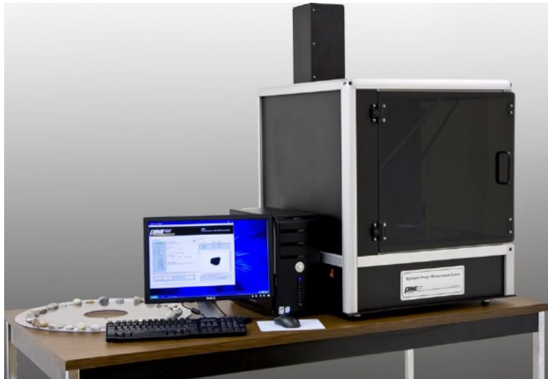
Figure 10 Second Generation Aggregate Imaging Measurement System (12)
