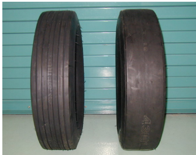
Figure 1 Ribbed (ASTM E501) versus Smooth Test Tire (ASTM E524) (3)
