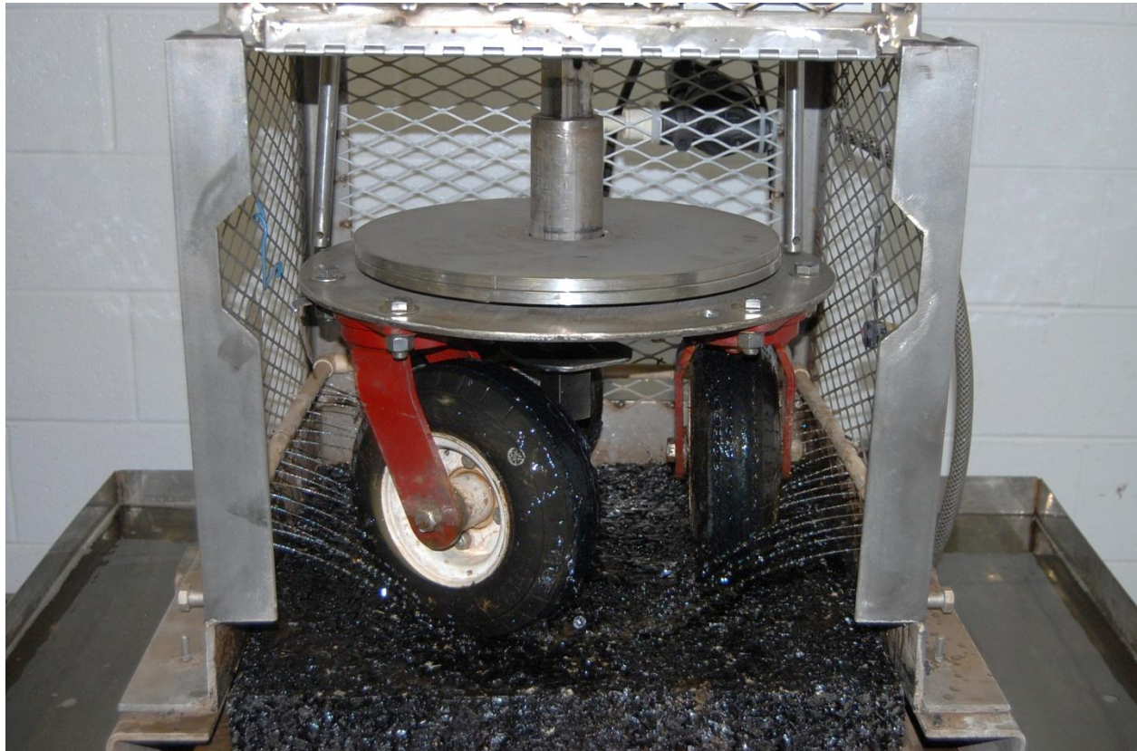
Figure 1 NCAT Three Wheel Polishing Device
