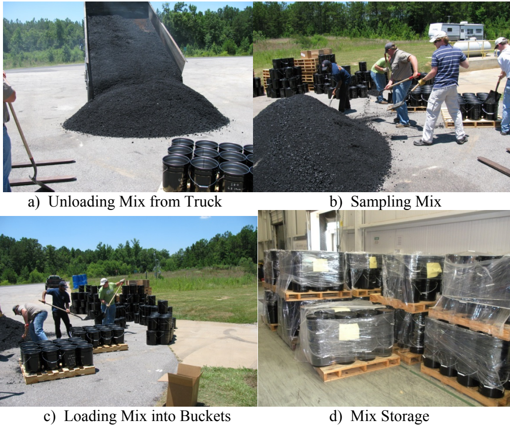
Figure 3.9 Mixture Sampling for Lab Testing
