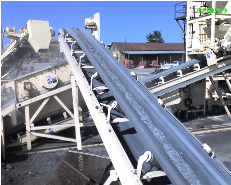
Figure 3.8 – TLA Pellets Fed Through RAP Feed System During Track Mix Production
