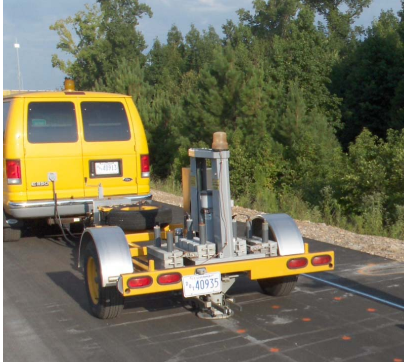
Figure 5.1 Dynatest Model 8000 FWD
