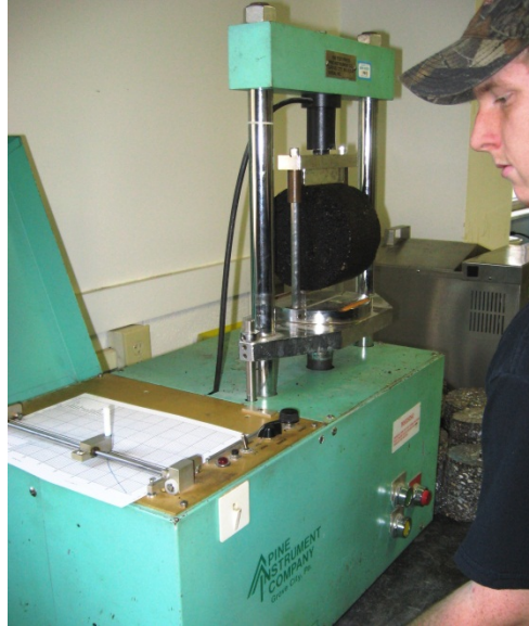
FIGURE 4.1 Pine Instruments Marshall Stability Press
