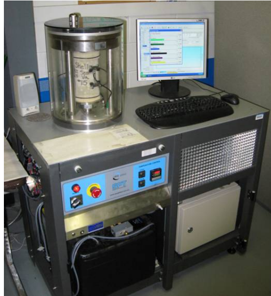
FIGURE 4.2 IPC Global Asphalt Mixture Performance Tester
