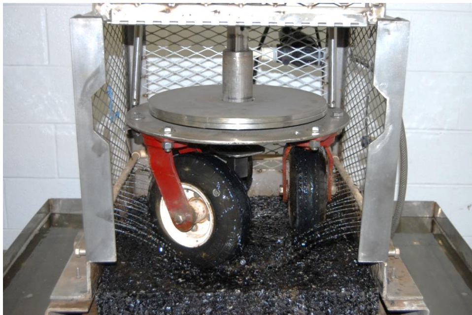
FIGURE 1 NCAT Three Wheel Polishing Device
