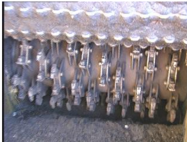
FIGURE 3 Cutting teeth inside grinding chamber (20)
