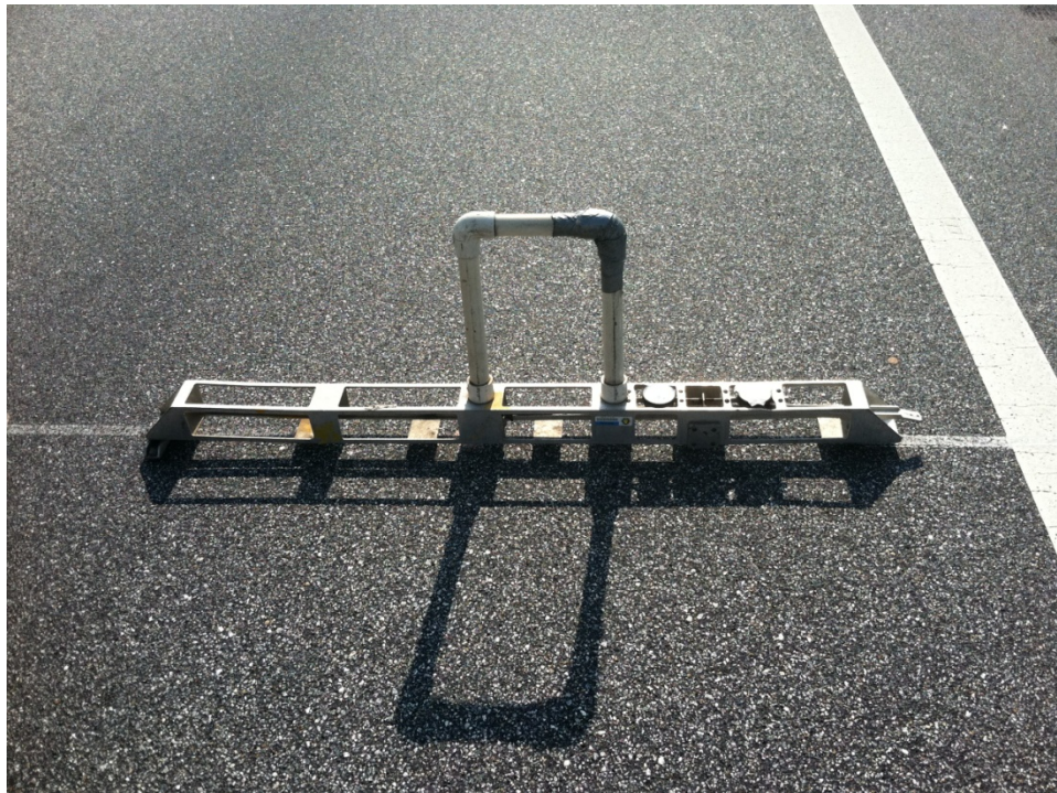
Figure 3.13 ALDOT Rut Depth Gauge Method
