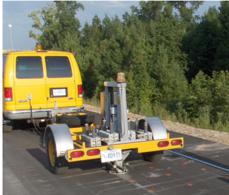
Figure 3.11 Falling Weight Deflectometer
