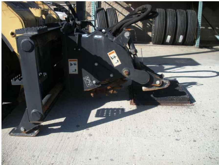
FIGURE 28 Attachment with Two Milling Drums for Milling and Micro-Milling Slabs.
