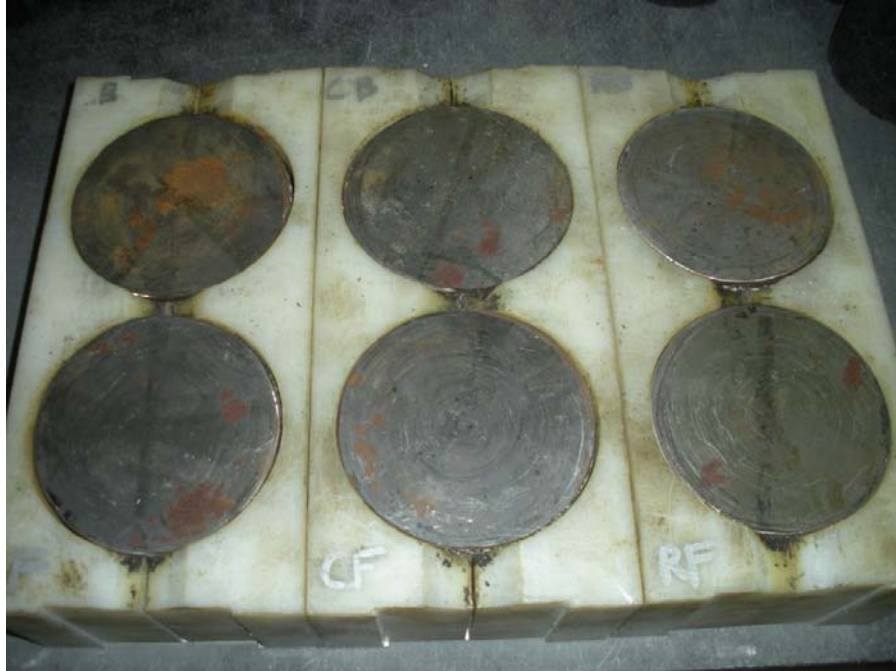
FIGURE 31 150-mm Steel Plates Placed on Specimens to Avoid Rutting in APA Testing.
