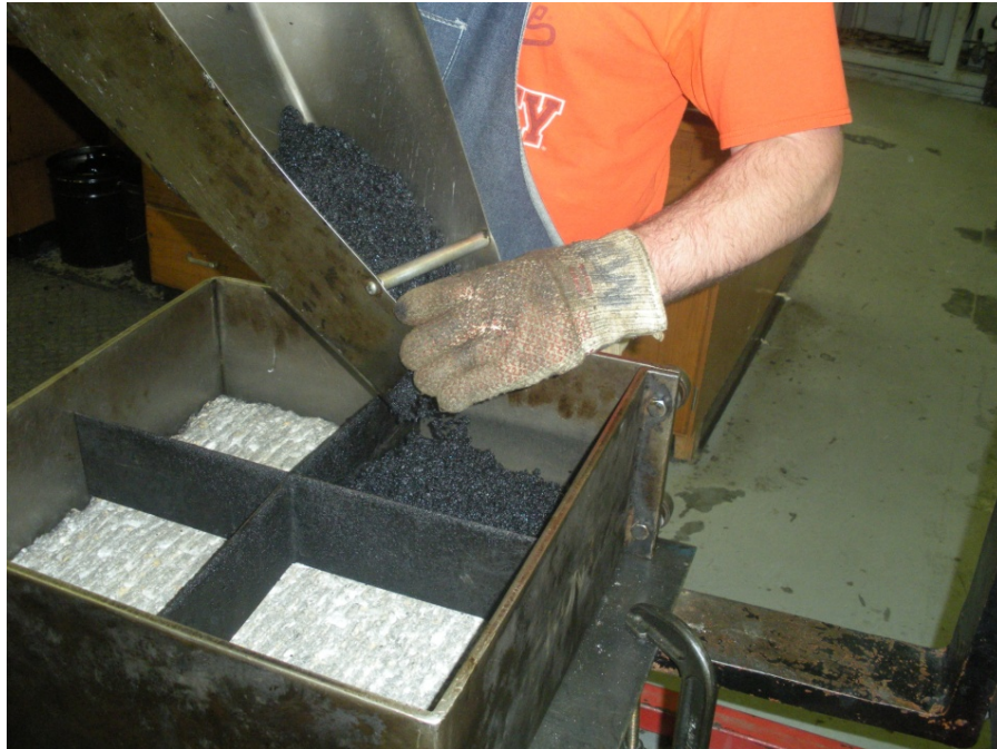
FIGURE 29 Compacting Top Layer on Non-Tacked Milled Underlying Layer Surface.
