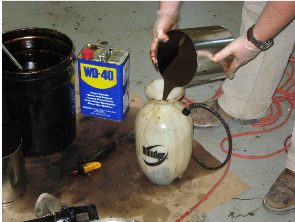
Figure 15 Sprayer used for Applying Tack Coat in Laboratory
