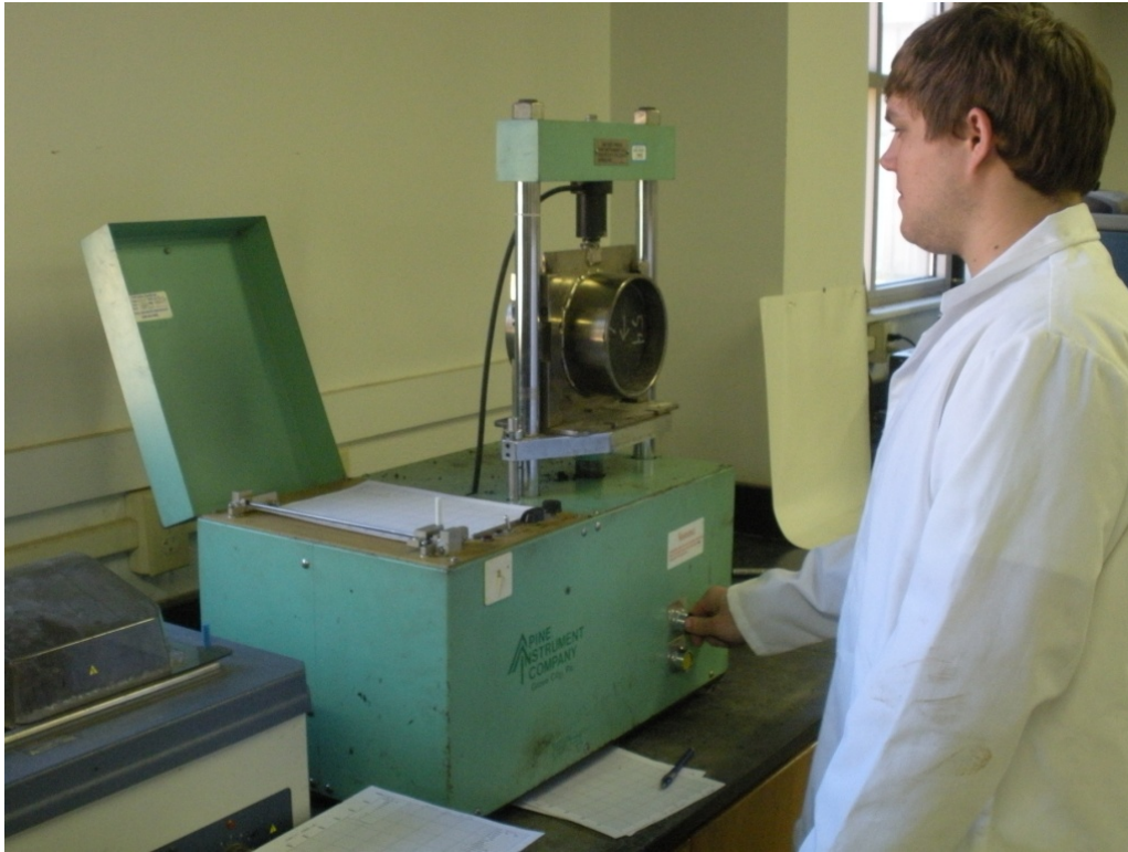
Figure 25 Conducting the Bond Strength Test
