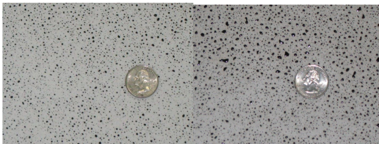
Figure 38 Emulsion Droplet Size – Nanotac Modified (left) and Control (right)
