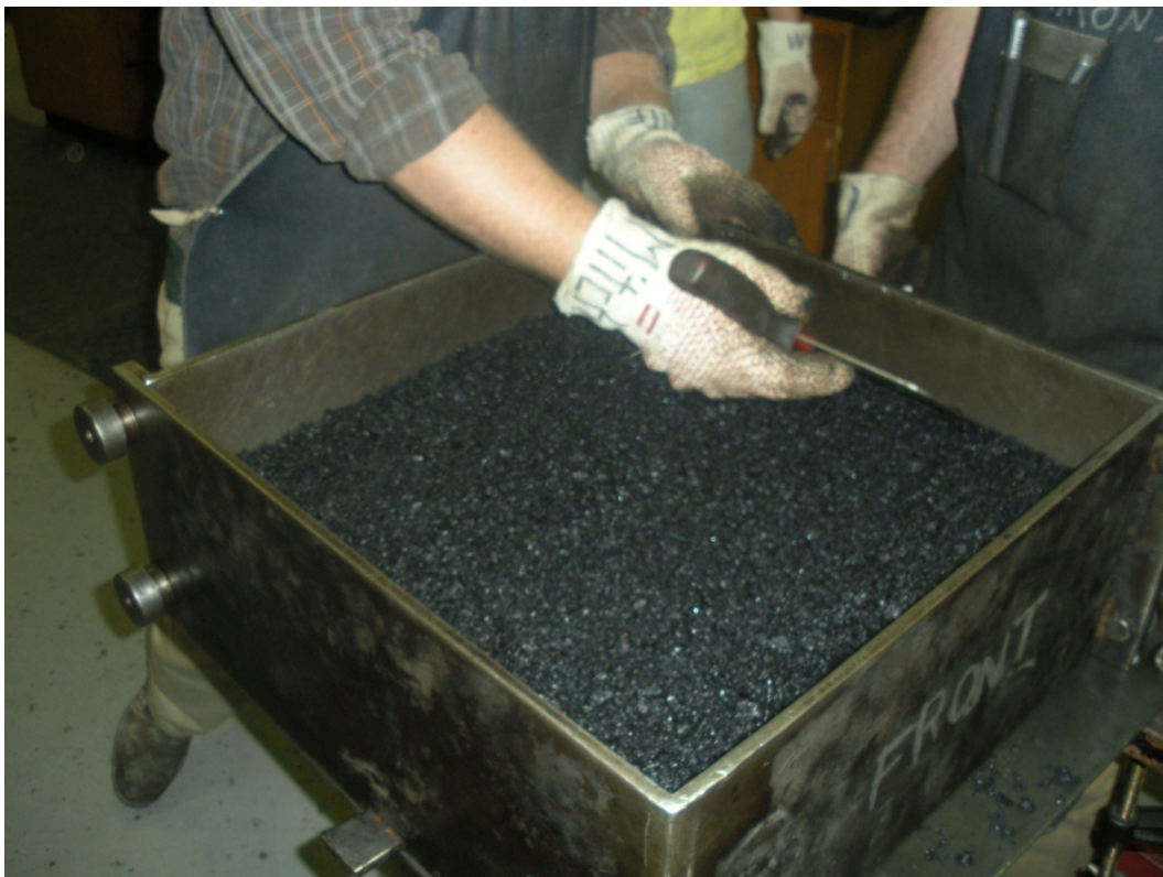
Figure 9 Leveling Mix in Mold
