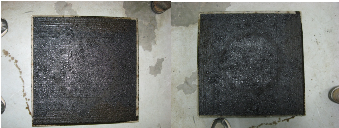
Figure 40 Slab with Control Emulsion both Before (left) and After (right) Tire-Pickup Experiment
