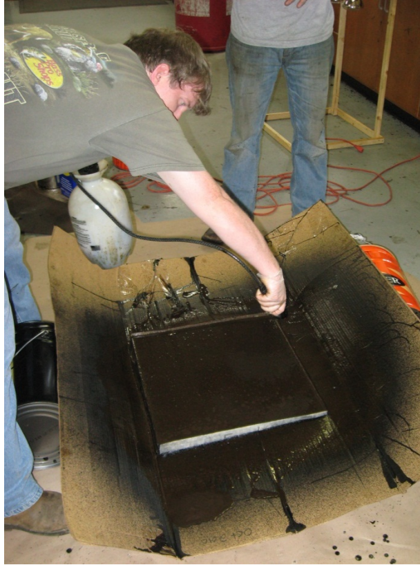
Figure 17 Device Used to Calibrate Application Overspray
