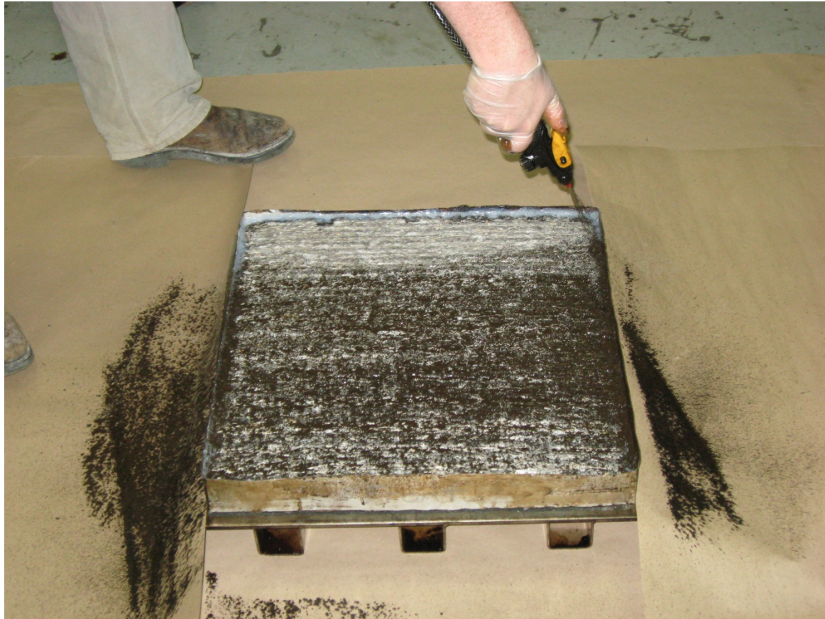
Figure 16 Spray Application of Tack Coat in Laboratory
