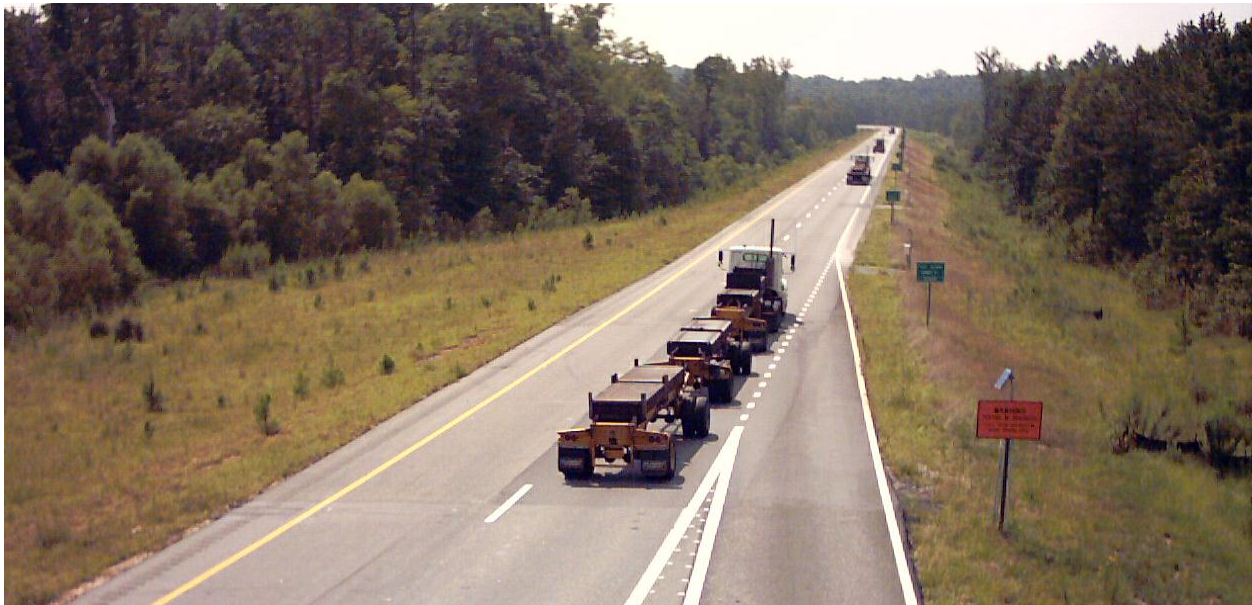
FIGURE 23 Application of Accelerated Damage on the NCAT Pavement Test Track
