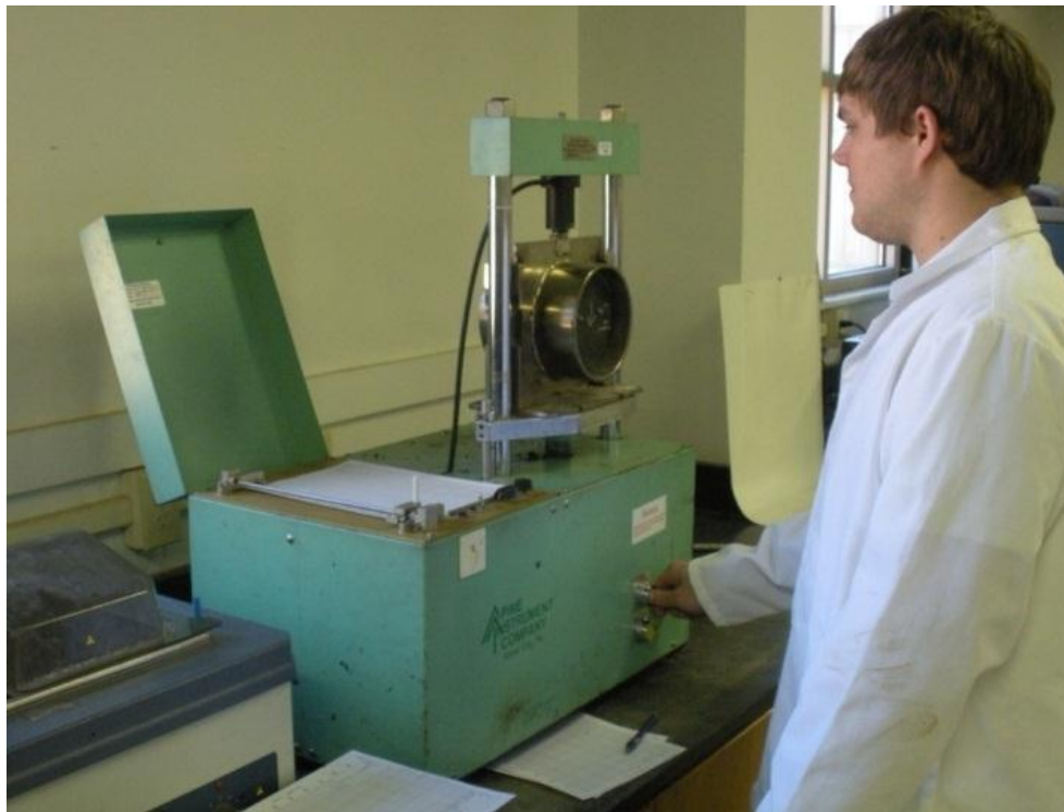
FIGURE 22 Bond Strength Testing In Progress
