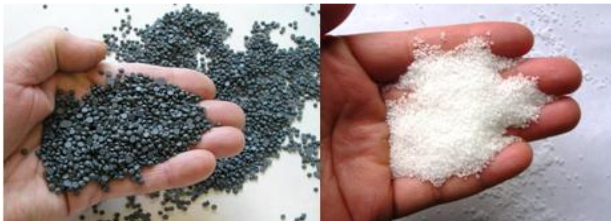
FIGURE 6 Thiopave Pellets and Compaction Aid (Timm, Tran, et al. 2009)
