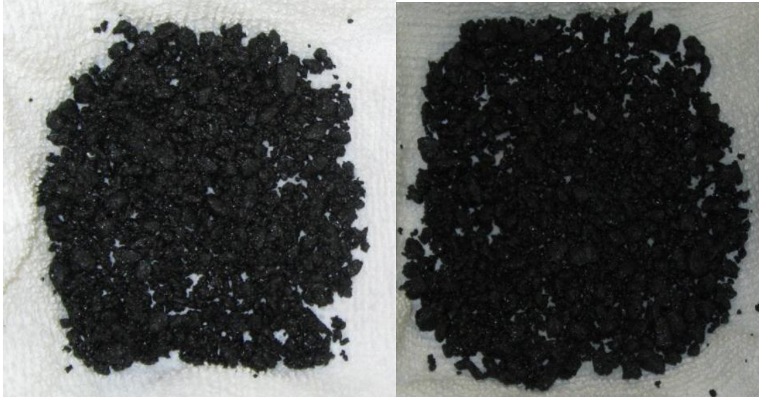
FIGURE 12 Loose Mix Samples Following Boiling Water Test - HMA (left) and WMA (right)
