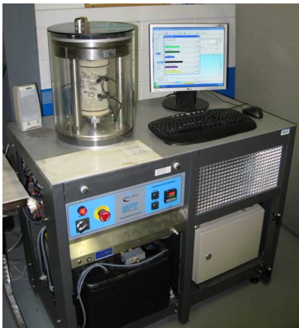
Figure 4.1 IPC Global Asphalt Mixture Performance Tester
