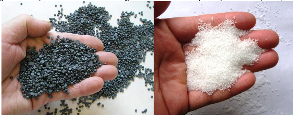
Figure 1.1 Thiopave Pellets and Compaction Aid (Timm et al., 2009)
