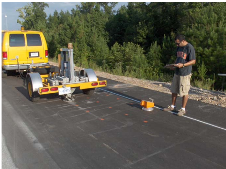
Figure 5.1 Dynatest Model 8000 FWD
