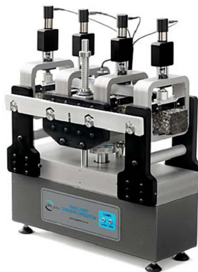
Figure 4.8 IPC Global Beam Fatigue Testing Apparatus
