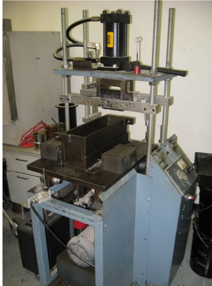
Figure 4.7 Kneading Beam Compactor
