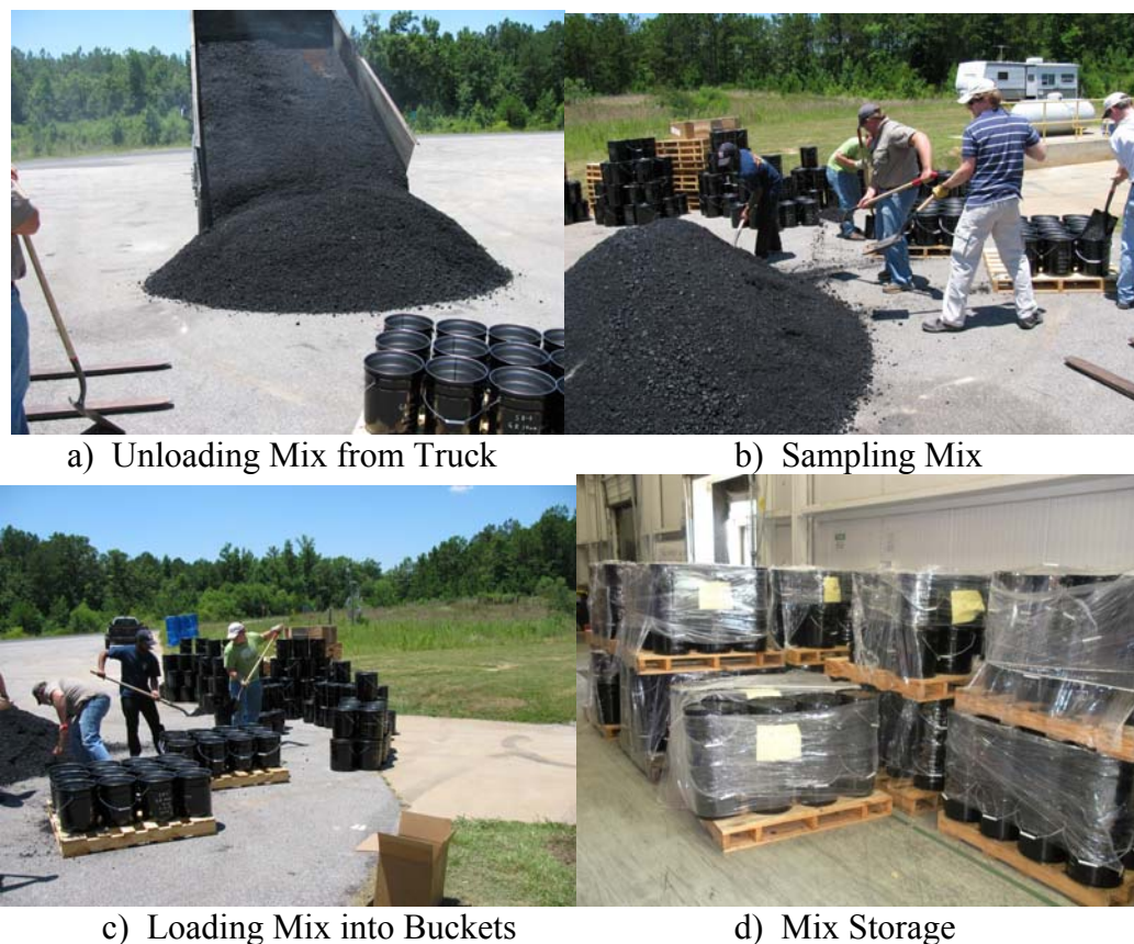
Figure 3.8 Mixture Sampling for Lab Testing
