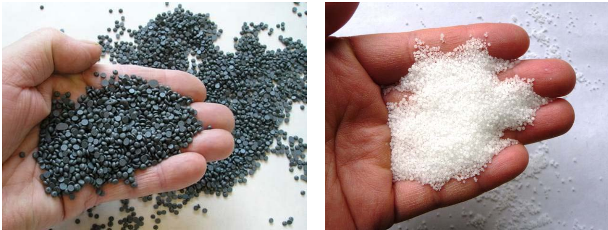
FIGURE 1 Modified Sulfur Pellets (left) and Compaction Agent (right) Used in Sulfur-Modified WMA.
