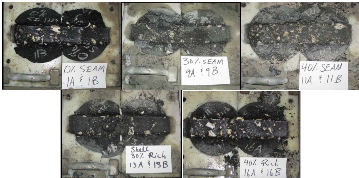
FIGURE 24 Tested Hamburg Wheel Tracking Specimens.
