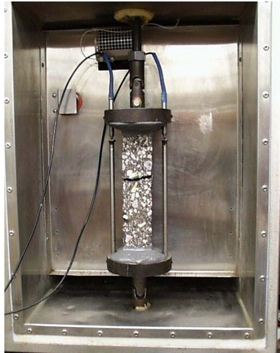
FIGURE 11 Thermal Stress Restrained Specimen Test.
