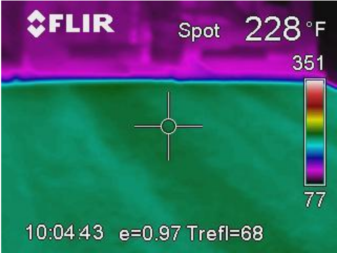
FIGURE 6 Thermal Image of Sasobit Mat (Picture courtesy of Becky Smith)
