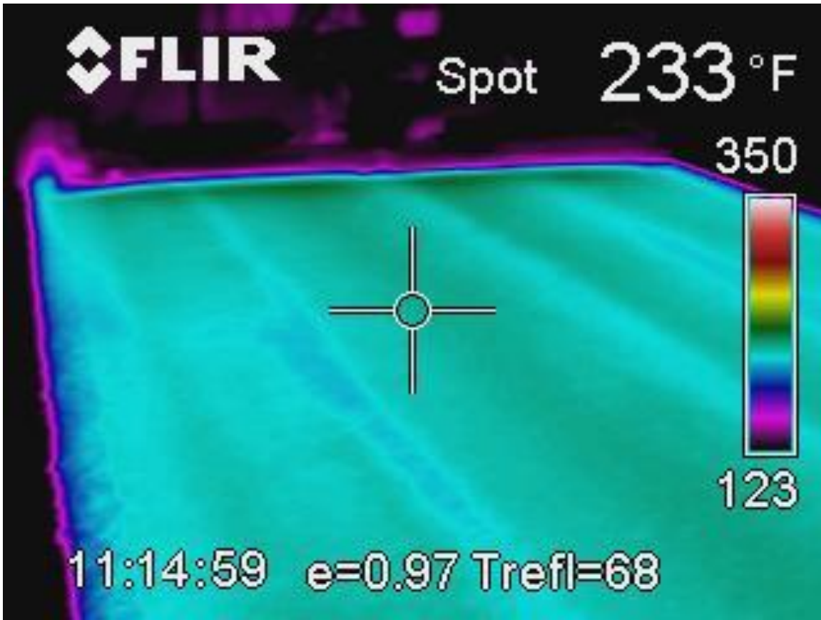
FIGURE 5 Thermal Image of Evotherm DAT Mat (Picture courtesy of Becky Smith)
