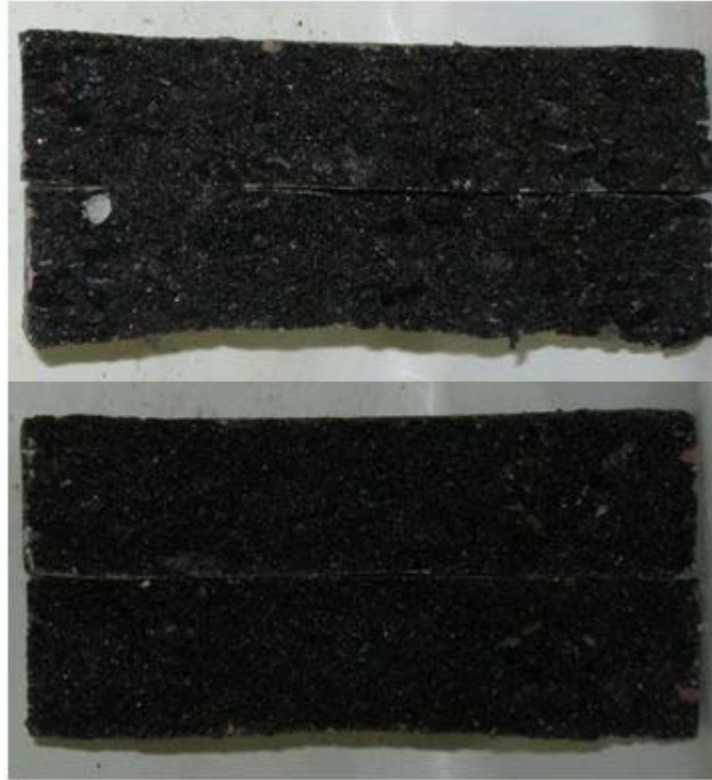
FIGURE 11 2 Year Cores, Control (Top) and Sasobit® (Bottom)
