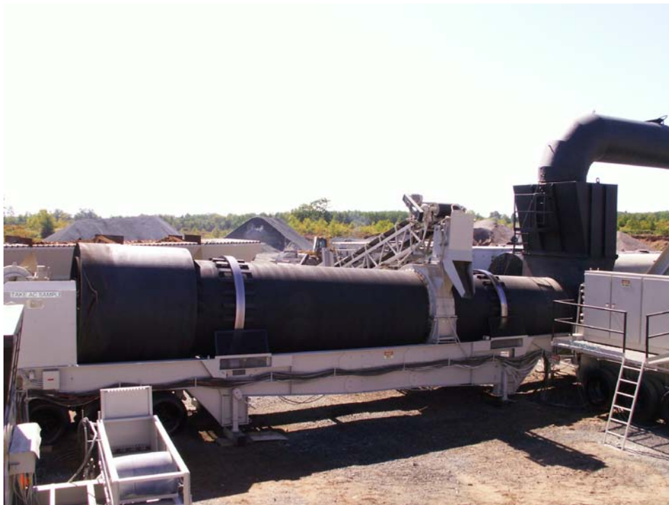
FIGURE 2 Payne and Dolan's Iron Mountain, MI Portable Asphalt Plant.
