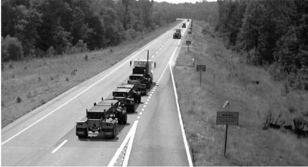
FIGURE 38 Triple trailers used to traffic the 2003 Track (42).
