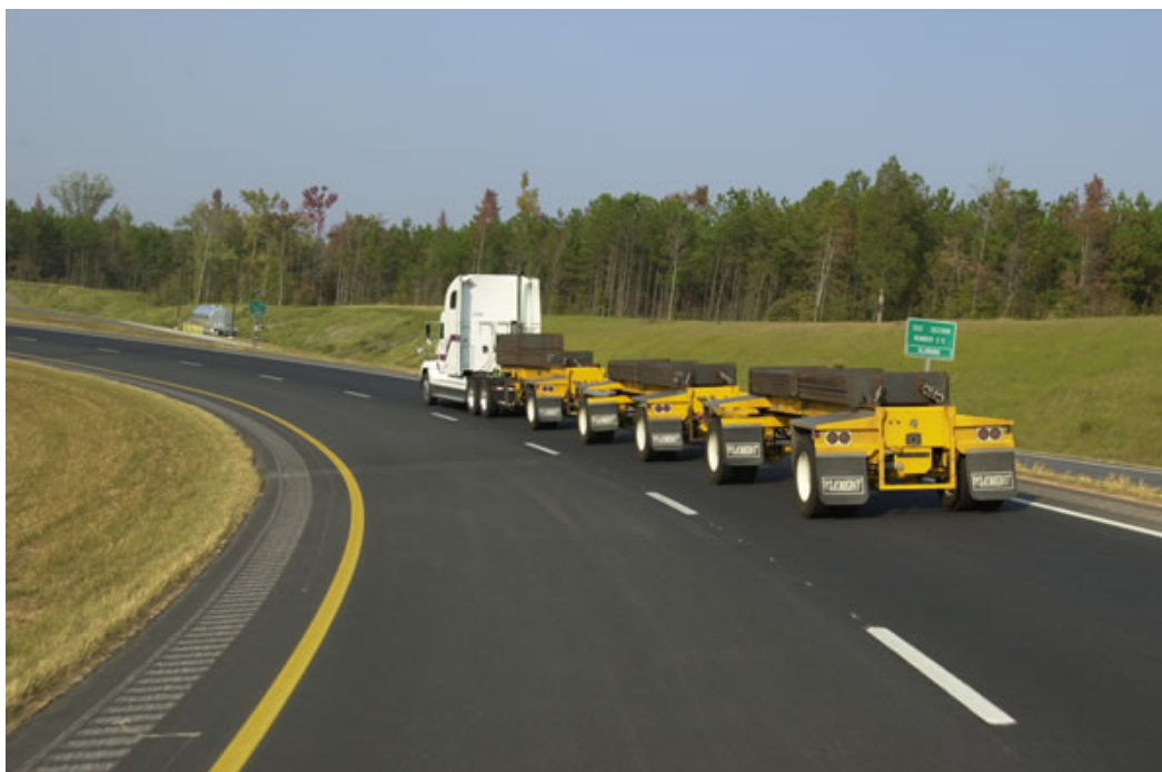
FIGURE 29 Triple trailer used for loading during the 2000 Test Track experiment.
