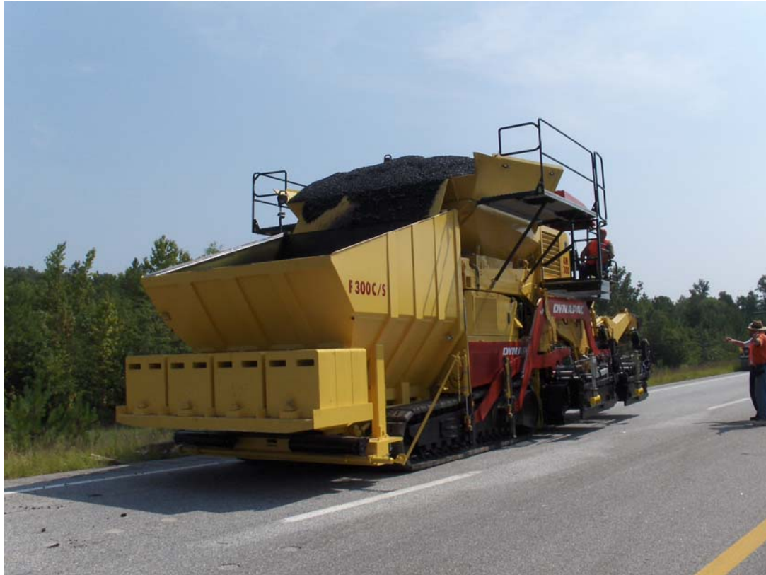
FIGURE 15 Twin layer paver that paved section N13 in 2006.
