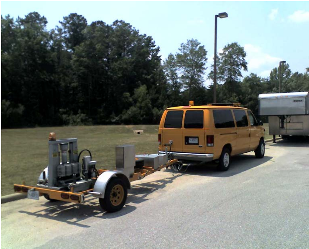
Figure 2.4 Dynatest 8000 Falling Weight Deflectometer.
