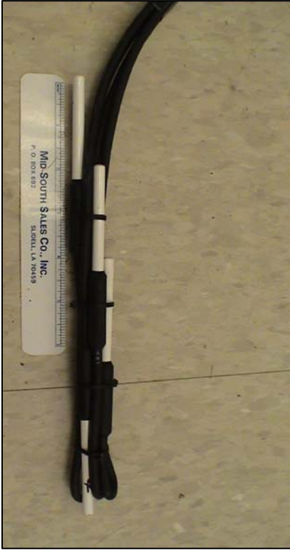
Figure 3.15 Typical Sub-Surface Thermistor Bundle Employed at the NCAT Test Track (after Priest and Timm “Fatigue,” 2006).
