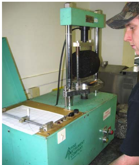
FIGURE 4.4 Pine Instruments Marshall Stability Press.
