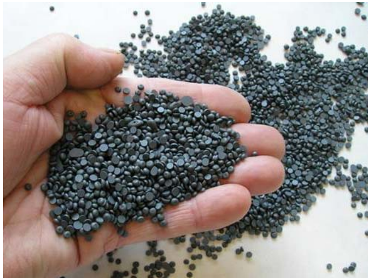
FIGURE 1.1 Shell Thiopave for Sulfur-Extended Asphalt Mixtures.
