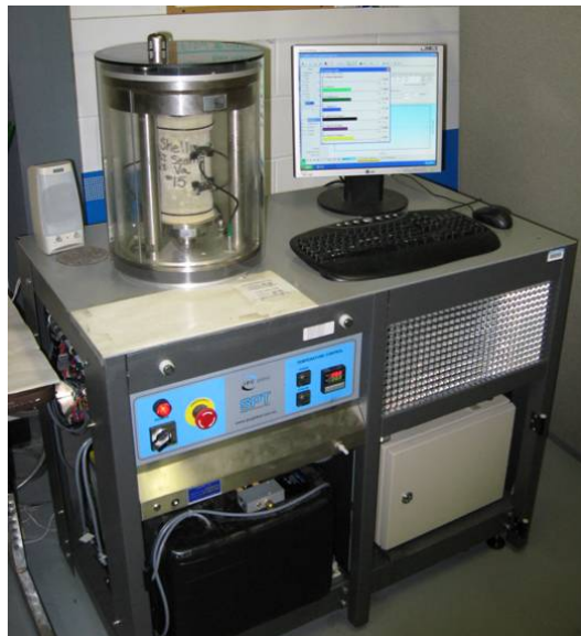
FIGURE 4.5 IPC Global Asphalt Mixture Performance Tester.
