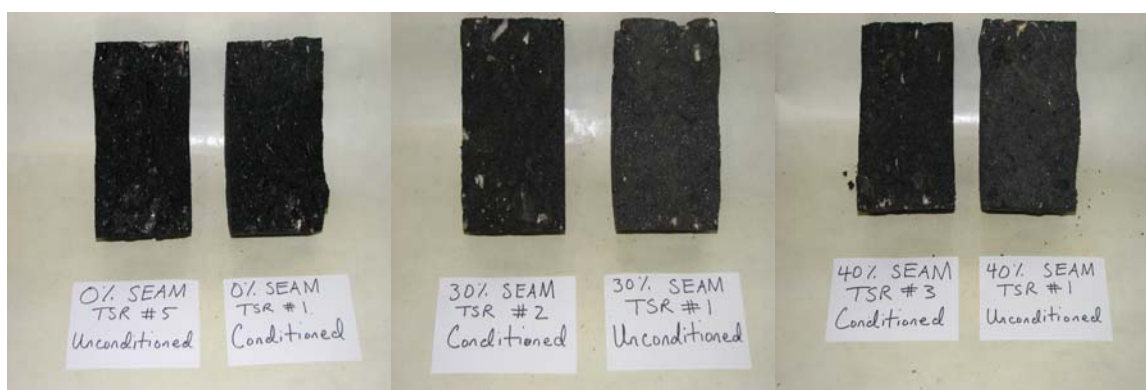
FIGURE 5.4 Broken TSR Specimens.
