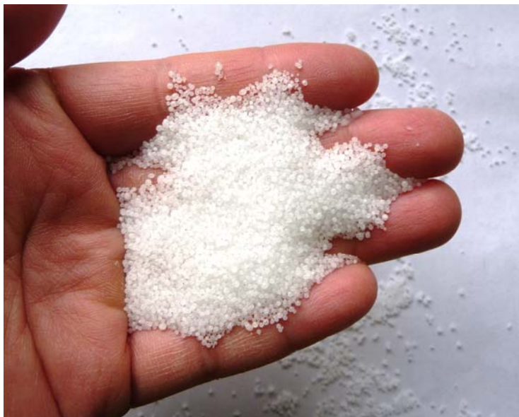
FIGURE 4.2 Compaction Aid Used for Thiopave Mixtures.
