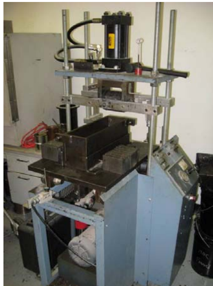
FIGURE 4.9 Kneading Beam Compactor.
