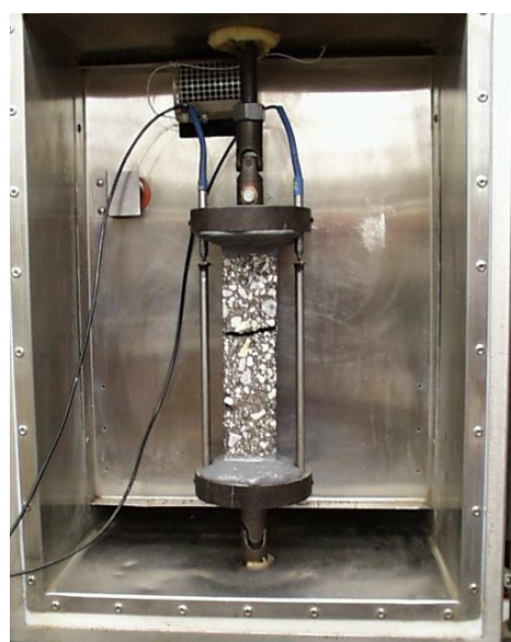
FIGURE 4.12 Thermal Stress Restrained Specimen Test.
