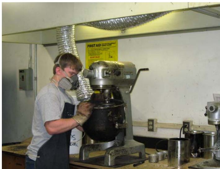
FIGURE 4.3 Mixing of Thiopave Mixture.
