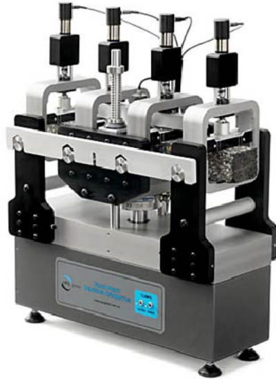
FIGURE 4.10 IPC Global Beam Fatigue Testing Apparatus.
