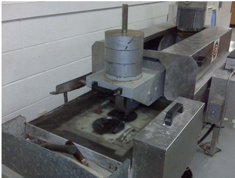
FIGURE 4.7 Hamburg Wheel-Tracking Device.
