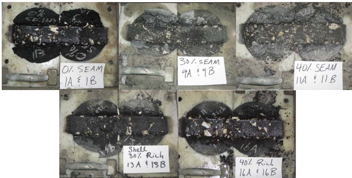
FIGURE 5.15 Tested Hamburg Wheel Tracking Specimens.
