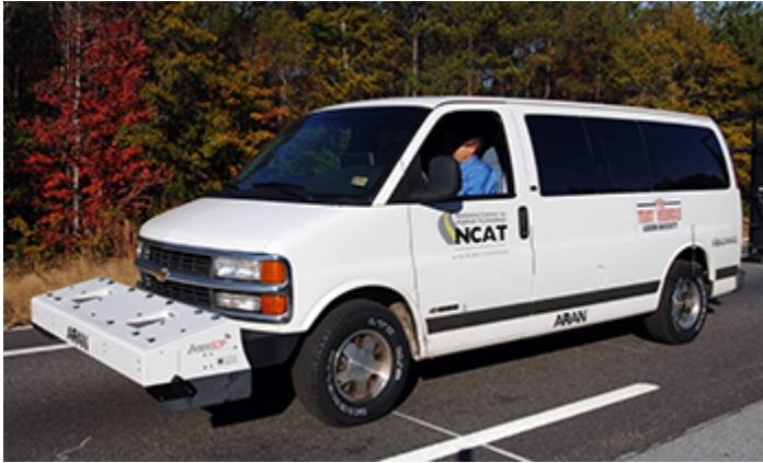
Figure 4. 5 ARAN Inertial Profiler at NCAT Test Track.
