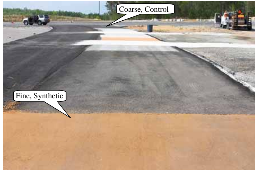
FIGURE 5 Twelve test sections constructed at plant site of NCAT Pavement Test Track.
