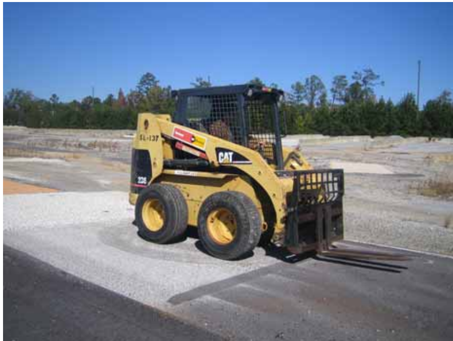
FIGURE 6 Skid steer loader for evaluating surface treatment durability.
