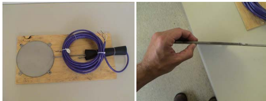
Figure 3.10. Geokon Earth Pressure Cell at the Test Track
