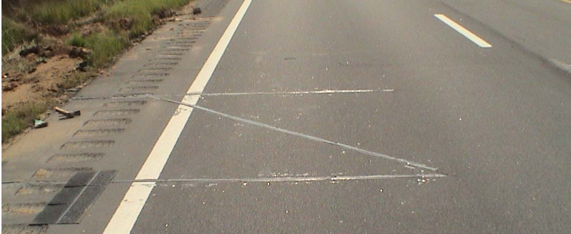
Figure 3.14. Axle Sensing Strips for Measuring Wheel Wander
