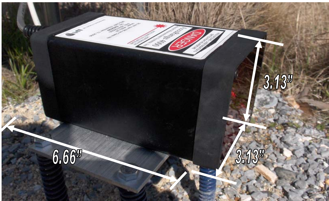
Figure 3.15. AR4000-LIR Distance Measuring Unit
