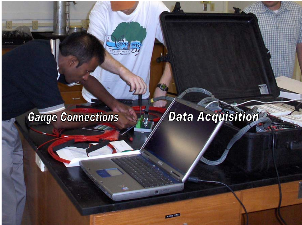
Figure 3.5. Connecting Asphalt Strain Gauges for Functionality Check
