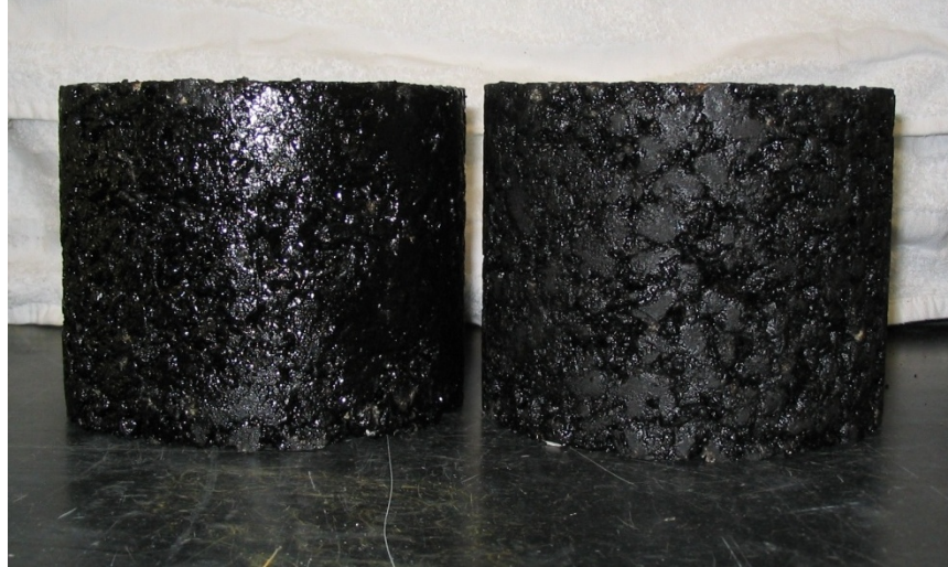
Figure 1. Stone Skeleton Asphalt Sample With (right) and Without (left) Mineral Fiber
