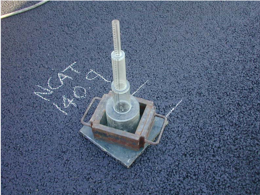
Figure 8. NCAT Field Permeameter
