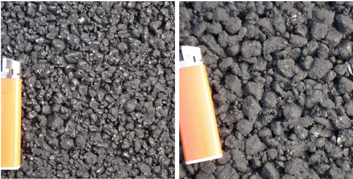
Figure 1: Surface textures of the OGFC (left) and PEM (right) mixtures.
