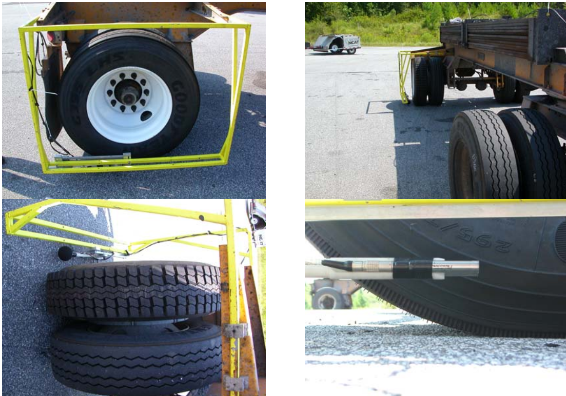
Figure 7. Sound intensity measurements with the triple trailer truck
