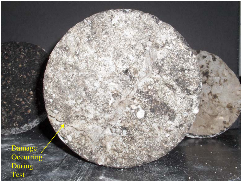
Figure 4.15 SMA Damage from Trench 2.
