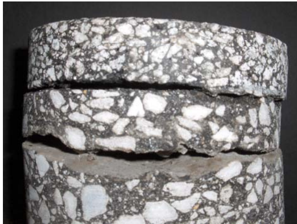
Figure 4.13 Extra Break in Core 2O1.
