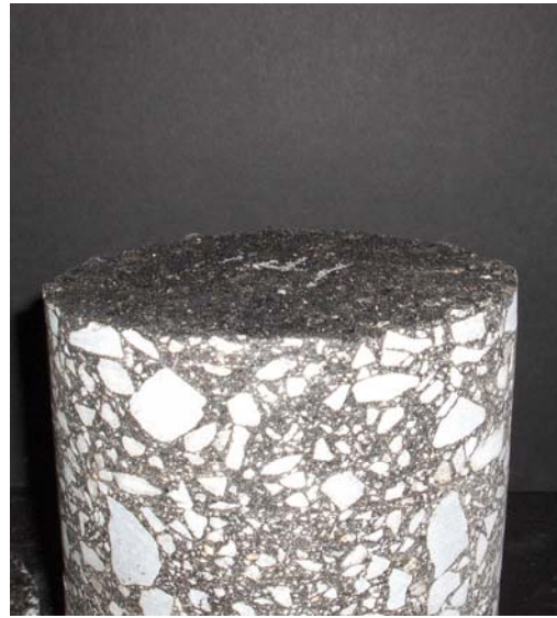
Figure 4.11 Clean Break of Core 1A1.
