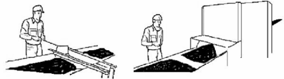
Reference Method Complete Cross-Section Removal by Stopped-Belt Sampling
