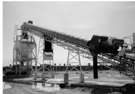
CLEAN SWEEP® Sampler Retro-fit Installation on a Truck Load-out Conveyor
