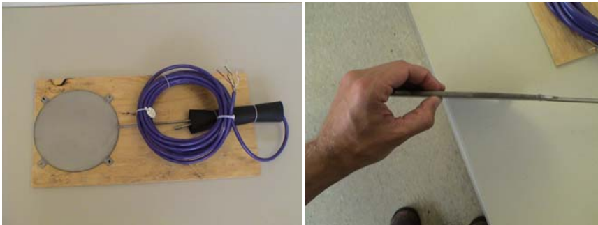
Figure 3.3 Geokon Earth Pressure Cell at the Test Track.
