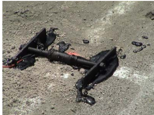
b) Finished Gauge
