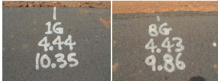
Figure 3.18 Wheelpath Markings for Cells N1 and N8.
