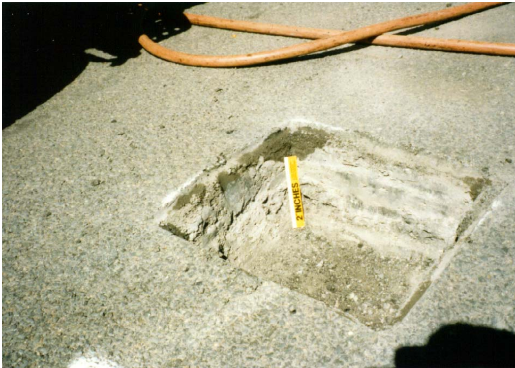
Figure 30. Test Hole Showing a Very Wet AC 14 Course Just Below the OGFC
