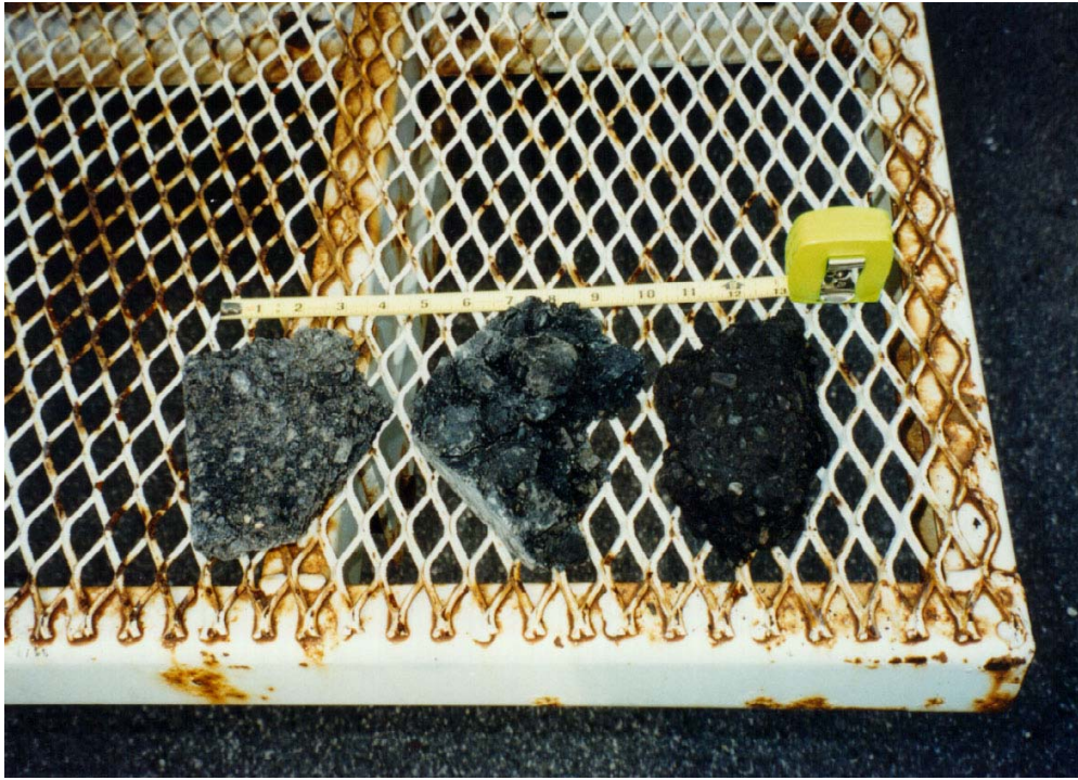
Figure 7. From Left to Right: New Gravel Wearing Course, Old Limestone Binder Course, and Old Gravel Wearing Course, From a Hole at MP 217.65
