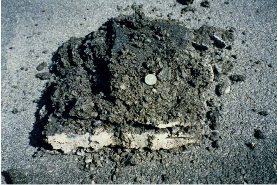
Figure 22. Bottom of Stripped B Mix Layer
