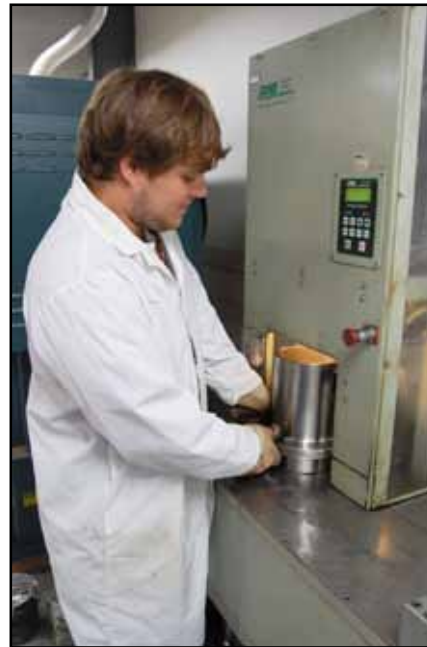
Figure 1 Compaction of an asphalt mixture in the Superpave Gyratory Compactor.
