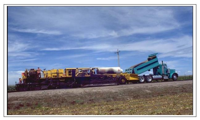
Figure 10. Hot In Place Recycling Method of Flexible Pavement
