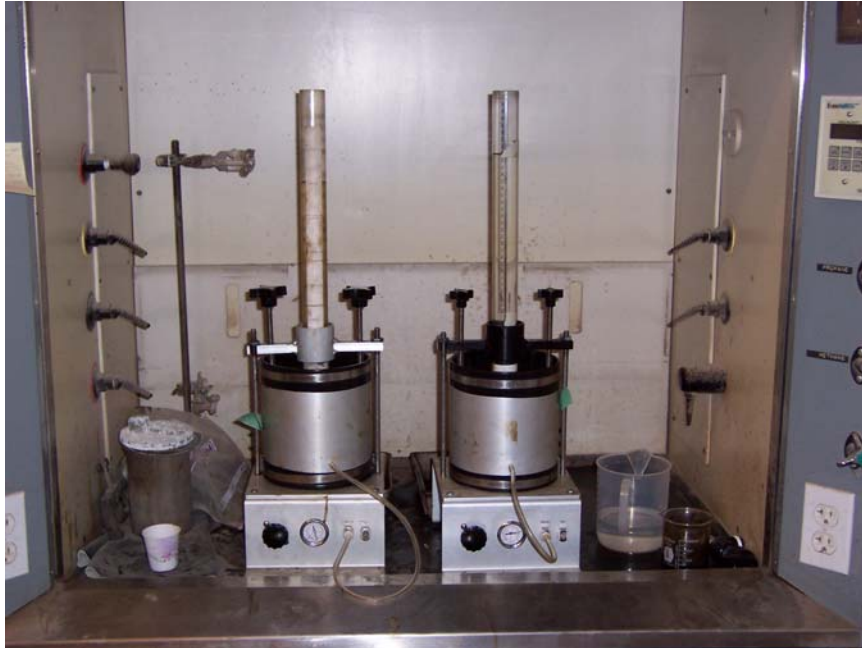
Figure 3-30 – Laboratory Permeameter Used for Testing (all testing was done in a fume hood due to the volatility of the kerosene)
