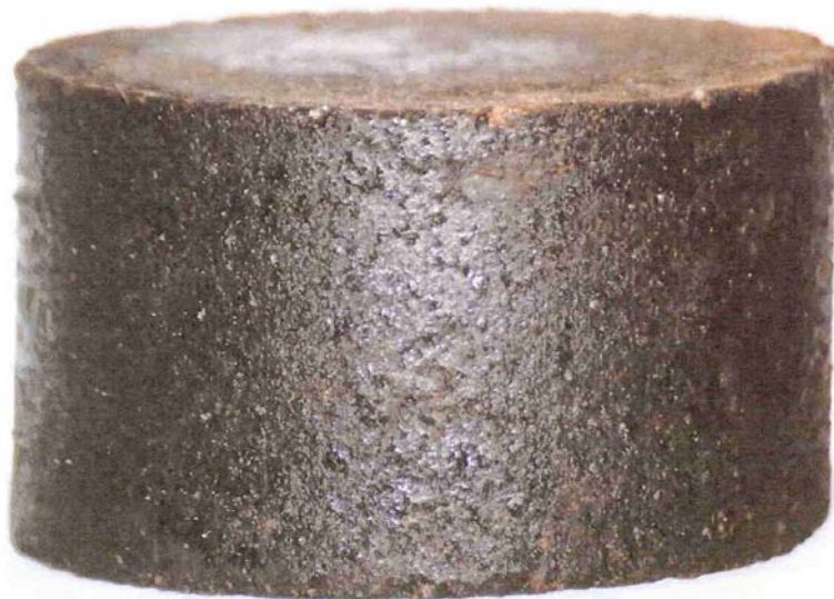
Figure 2-22 – Fuel Soaked StellaFlex Fuel Resistant Binder/HMA Specimen
