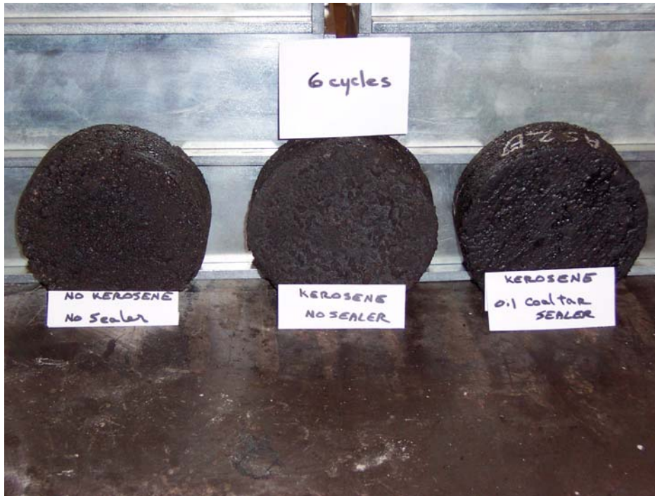
Figure 3-5 Samples after Abrasion Testing with Wire Brush
