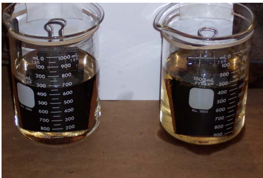
Figure 3-26- Samples placed in the fluid (the sample on right is kerosene, and the sample on left is jet fuel)
