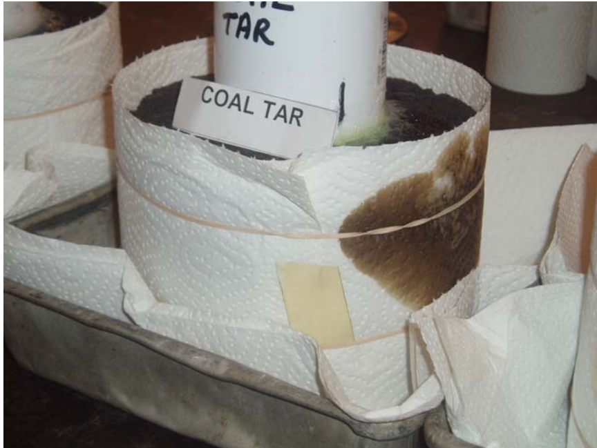
Figure 3-14 – Coal Tar at 30 minutes:
