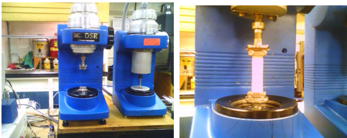
Figure 2-18 – DSR Dynamic Creep Setup
