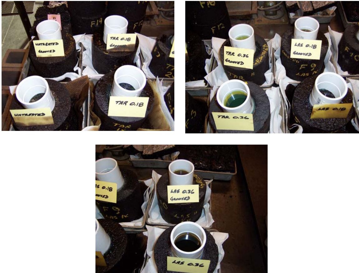
Figure 3-22 - Kerosene Level at Two Hours
