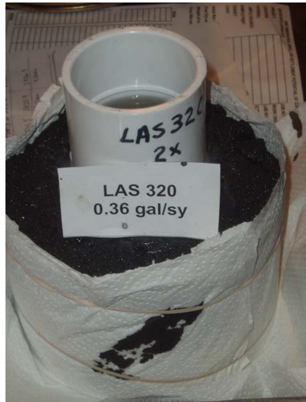
Figures 3-18 and 3-19 – LAS 320 with 0.36 gallons per sq yd.
