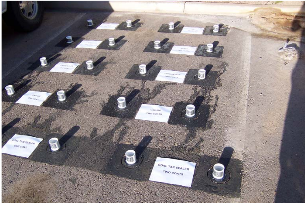
Figure 3-32 – Layout Of Field Test Sections
