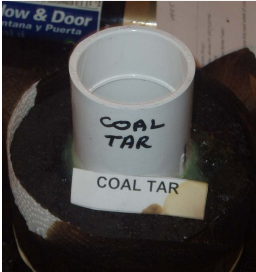
Figure 3-15 – The coal tar test after four hours.
