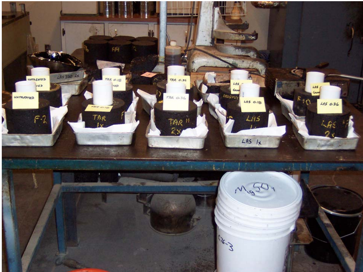
Figure 3-20 - Permeability Test Set Up
