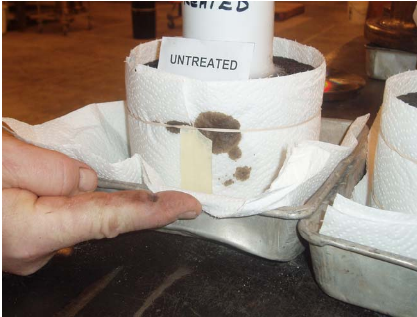
Figure 3-12 – Untreated at Five Minutes: Note seepage through side of specimen.
