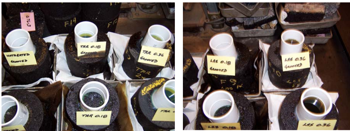
Figure 3-23 - Kerosene Level at Three Hours
