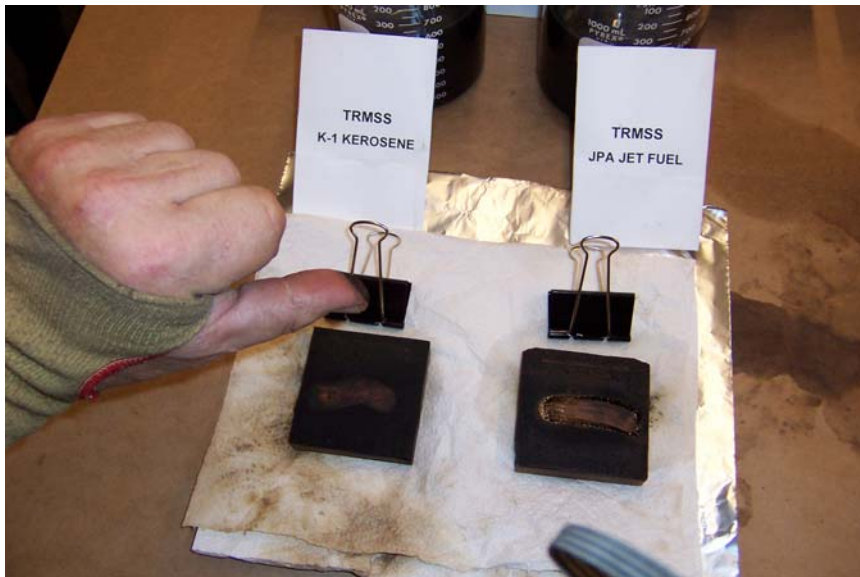
Figure 3-28 – Thumb Test on TRMSS Sealer
