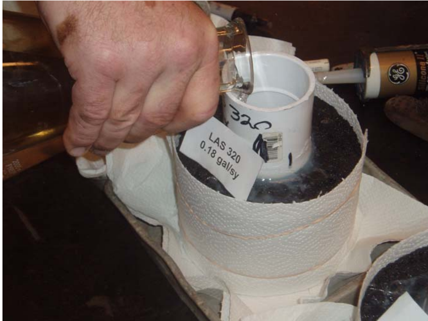
Figure 3-11 – Kerosene Being Poured into the PVC Pipe Coupler
