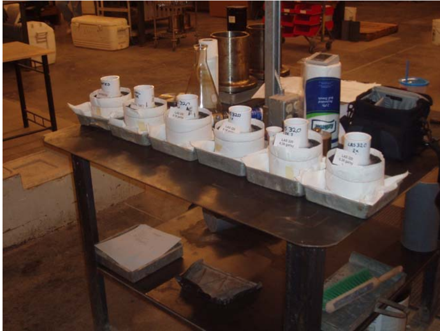
Figure 3-10 - Specimens Ready for Testing
