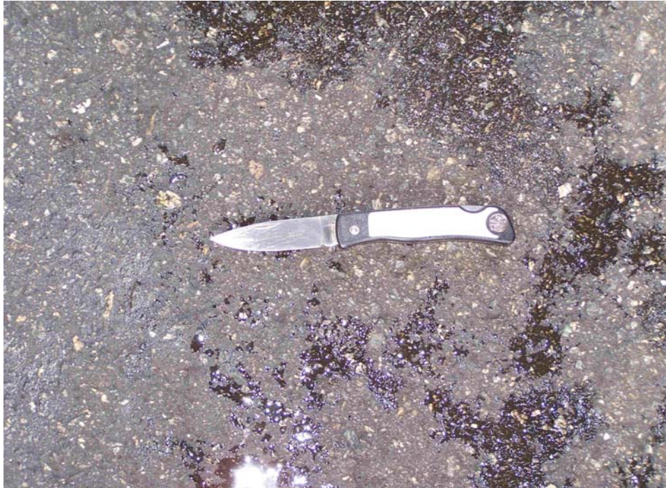
Figure 2-27 – Petroleum Contaminant on the SP FR 12.5 mm (fine).
