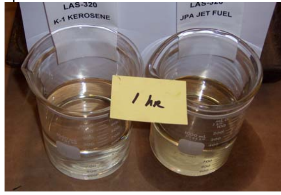
Fuel after removal of coated coal tar test specimen
