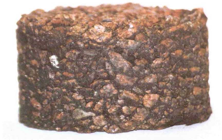
Figure 2-21 – Fuel Soaked Neat Binder/HMA Specimen.
