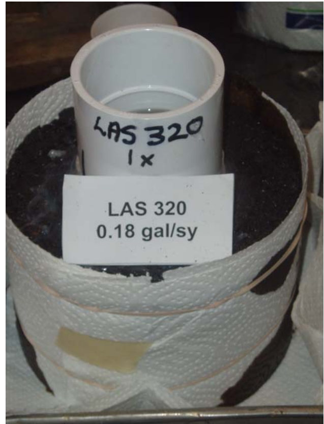
Figures 3-16 & 3-17 – LAS 320 with 0.18 gal/sy after four hours:
