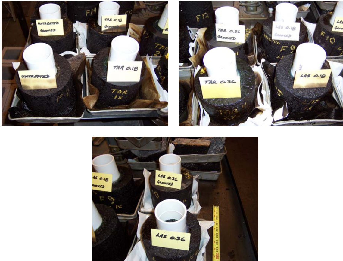
Figure 3-24 - Kerosene Level at Four Hours
