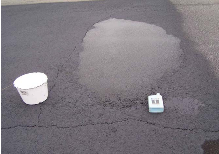
Figure 2-7 - Simulated Petroleum Spills on CarbonPlex Seal Coat.
