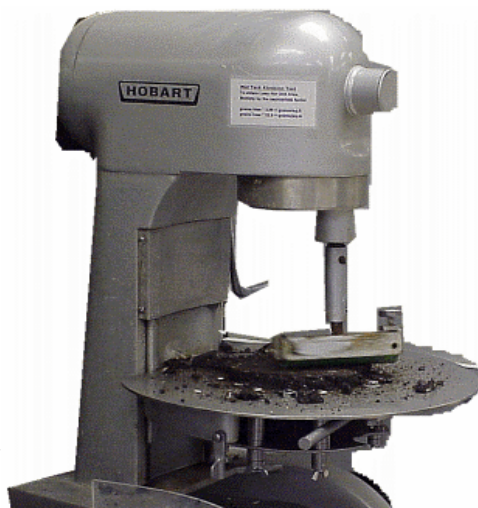
Figure 3-3 – Setup for Abrasion Test with Pneumatic Tube
