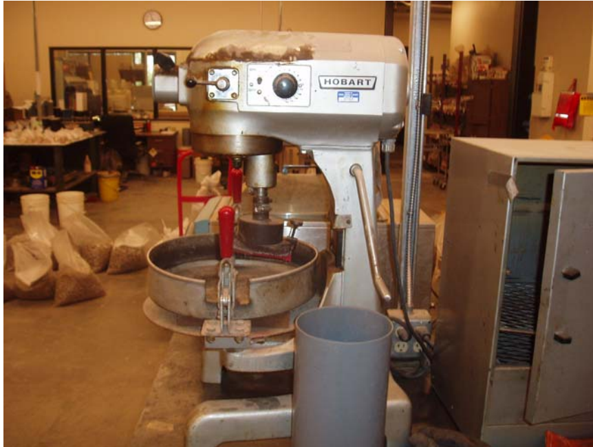
Figure 2-20 – Set up for Wet-Track Abrasion Test
