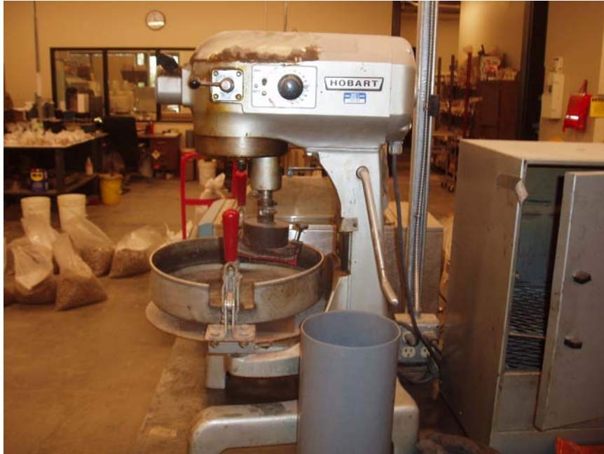
Figure 3-6 – Set up for Wet-Track Abrasion Test
