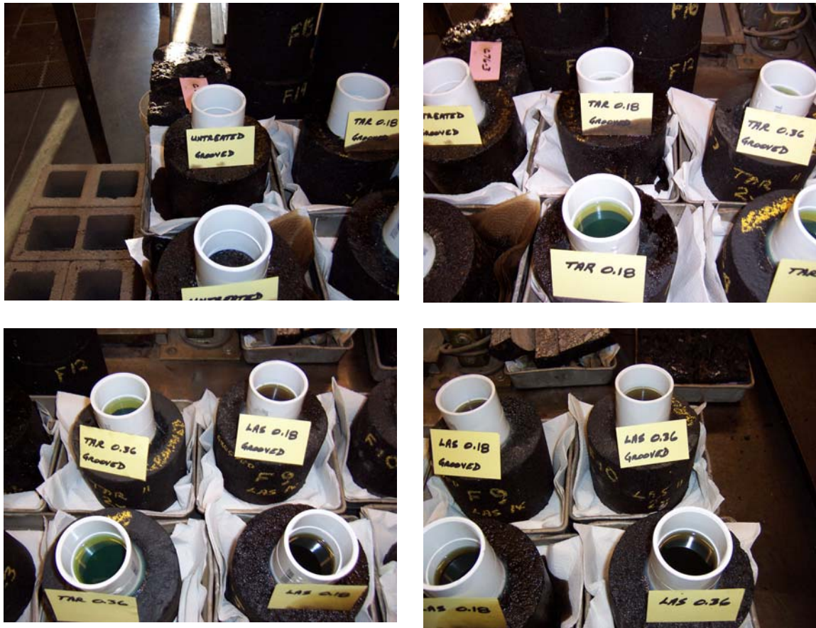
Figure 3-21 - Kerosene Level at One Hour
