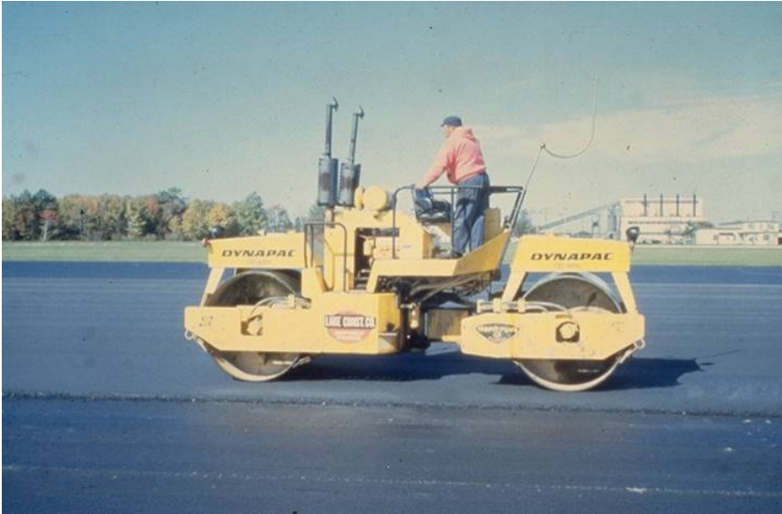
Figure 14.3 – Vibratory steel-wheel roller
