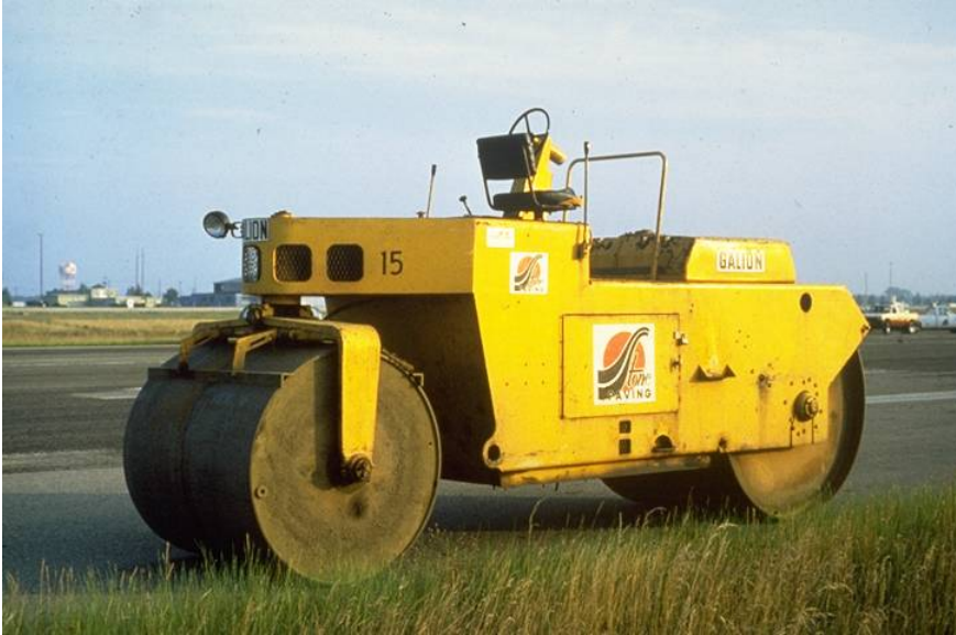
Figure 14.1 – Static steel-wheel roller
