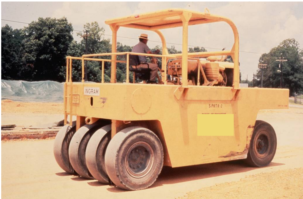
Figure 3.6 – Example of a rubber-tired pneumatic roller
