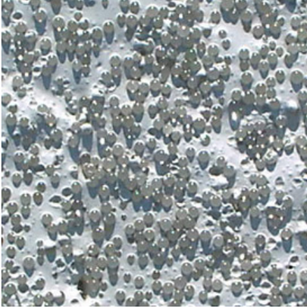
Figure 17.4 – Magnification of retroreflective glass beads embedded in marking paint (photo credit: Swarco)
