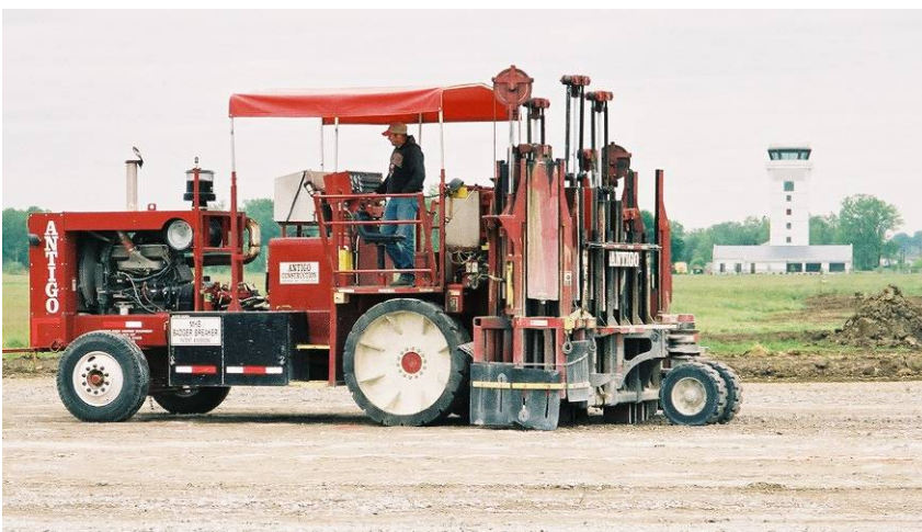
Figure 5.2 – Multiple head breaker (courtesy of Asphalt Institute)
