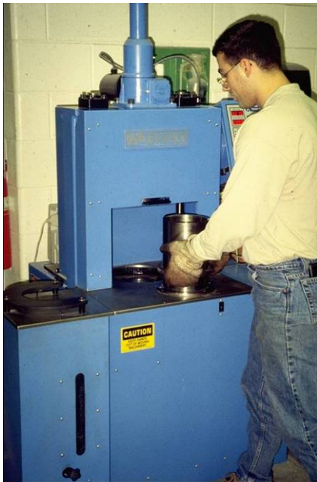
Figure 7.9 – Typical Superpave gyratory compactor.
