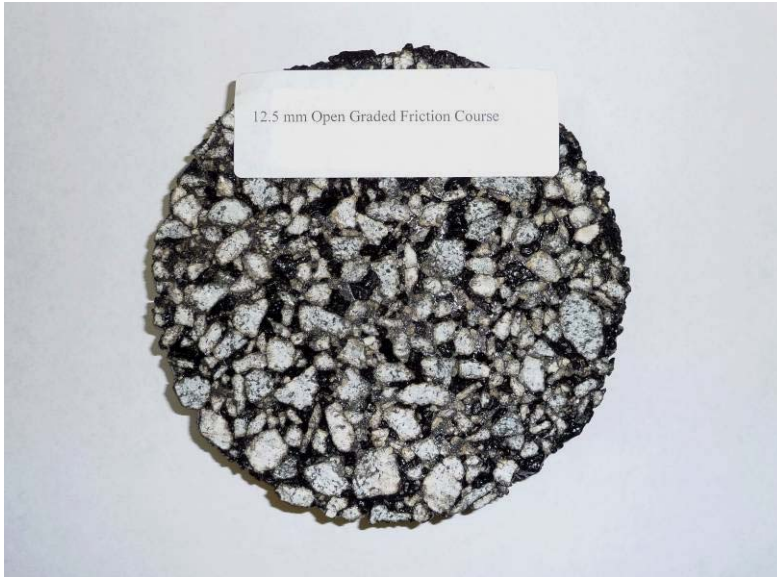
Figure 6.3 – Open-graded friction course
