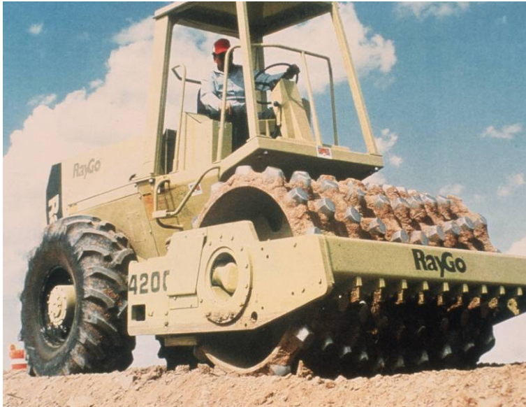
Figure 3.5 – Example of a sheepsfoot roller
