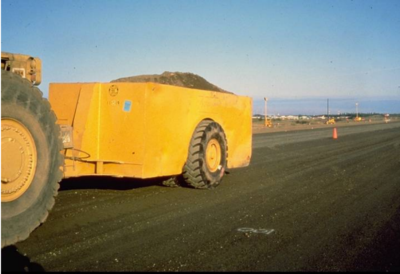
Figure 4.1 – Typical airfield proofroller
