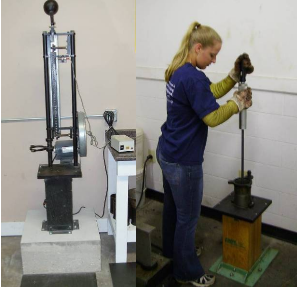
Figure 7.6 – Automatic Marshall hammer (left) and manual hammer (right)
