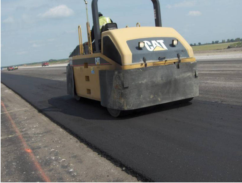
Figure 14.2 – Rubber-tire roller with skirts
