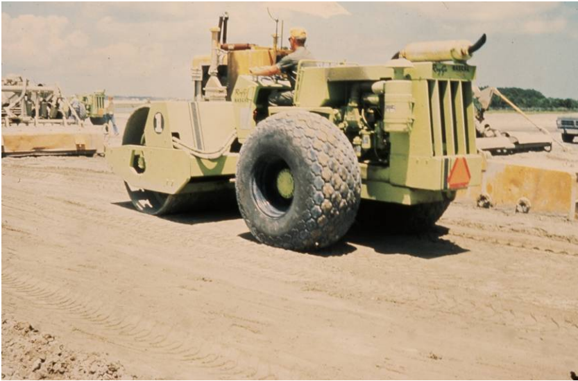
Figure 3.4 – Example of a vibratory steel-wheel roller
