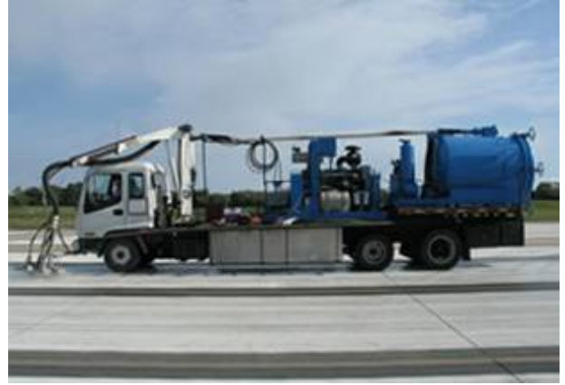
Figure 17.9 – High-pressure waterblasting truck (photo credit: D. Spiedel)
