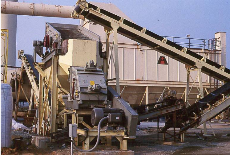
Figure 19.1 – In-line crusher and screening unit on RAP feed system
