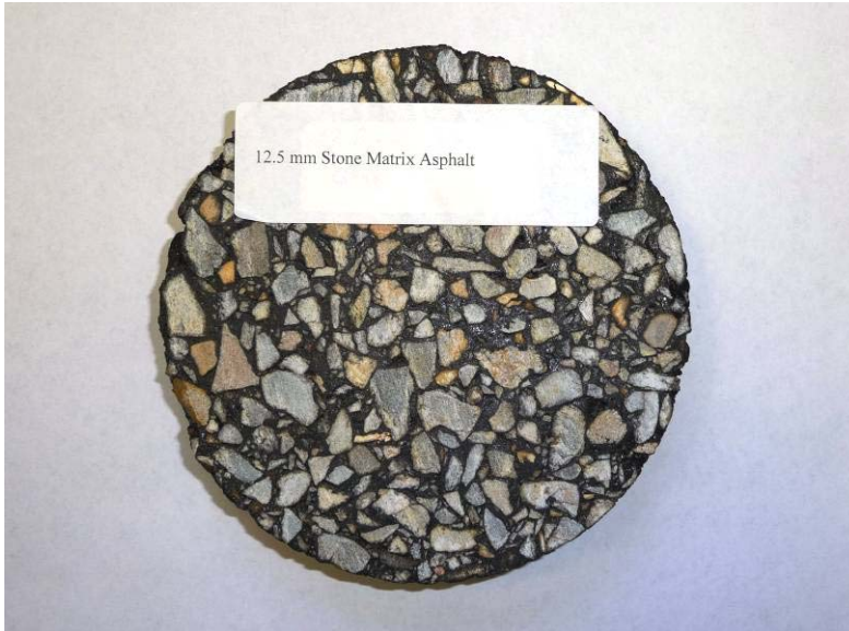
Figure 6.2 – Stone matrix asphalt mixture
