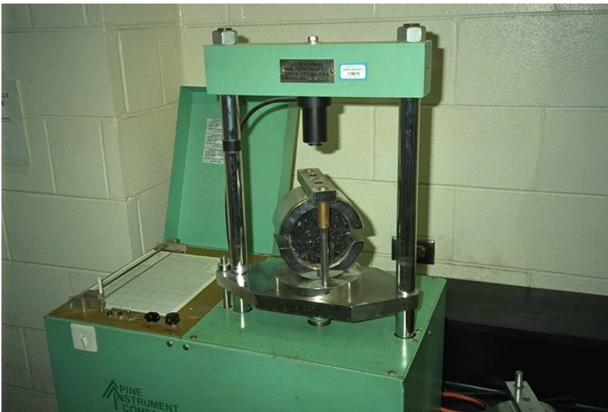
Figure 7.7 – Marshall stability and flow equipment
