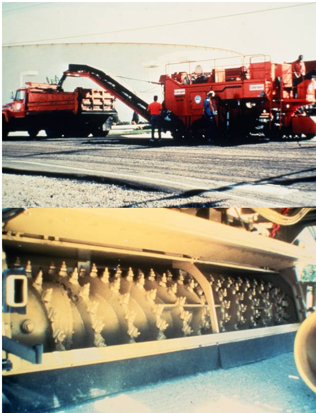
Figure 11.4 – Typical milling machine and drum with milling teeth
