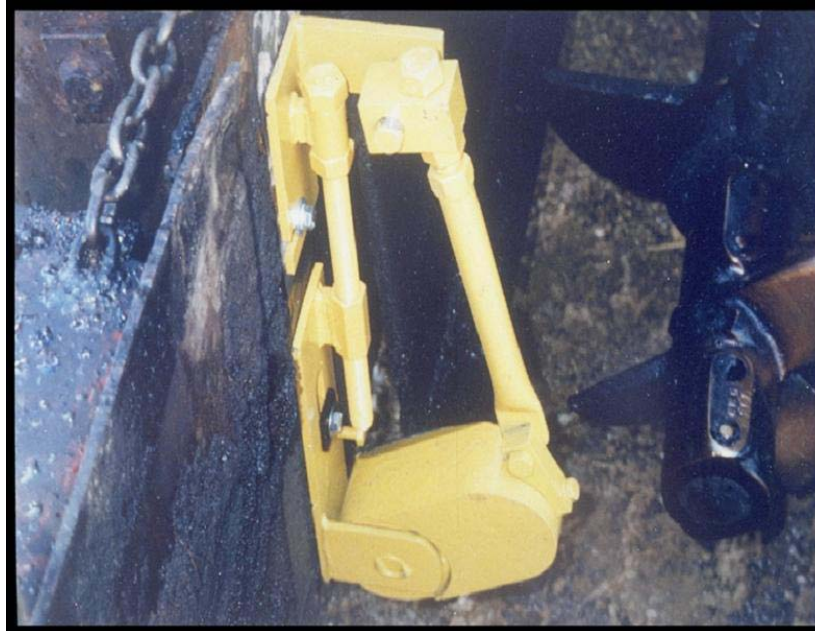
Figure 28. Joint maker attached to the side of the screed at corner
